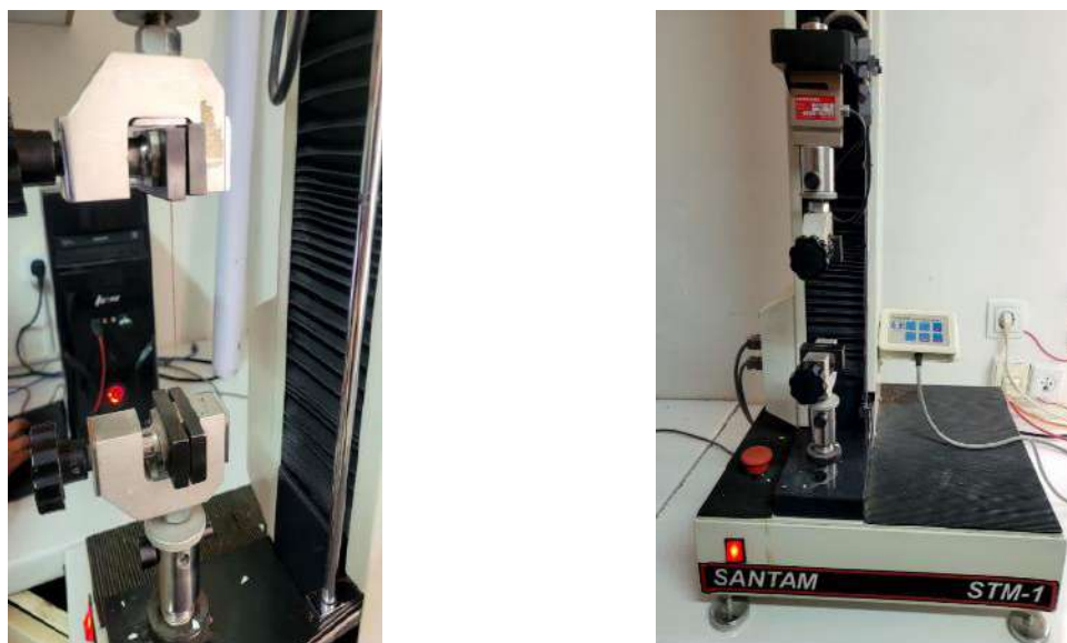
Fig. 3. Tensile test of date fibers with Bongshin device to determine tensile strength
