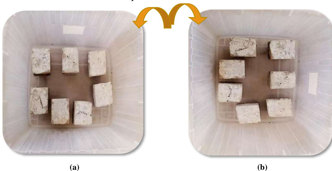
Fig. 4. 100 × 100 × 100 mm concrete cubes coated with transparent epoxy partially immersed to a depth of 5 mm at one end for varieties of time intervals: a) 7 concrete cubes immersed in water, first part; and b) 7 concrete cubes immersed in water, second part
