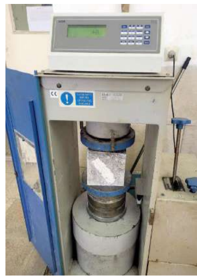
Fig. 7. The failure of the cube specimen with the compressive strength device, and the specimen broken with palm fibers
