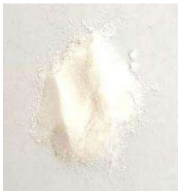
Fig. 6. VMA (solidifier and controller of concrete rheology)
