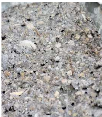
Fig. 8. Failure of the cylindrical test piece with the Brazilian device and the test piece broken with palm fibers
