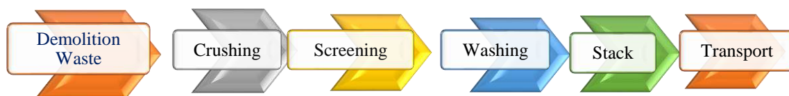
Fig. 2. Process for production of recycled concrete aggregate
