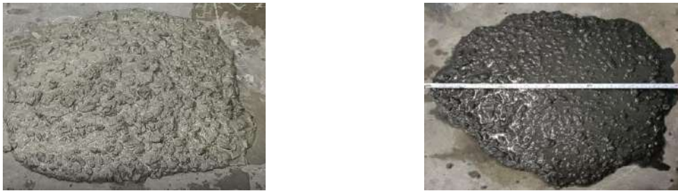
Fig. 6. Slump flow test on self-compacted recycled aggregate concrete
