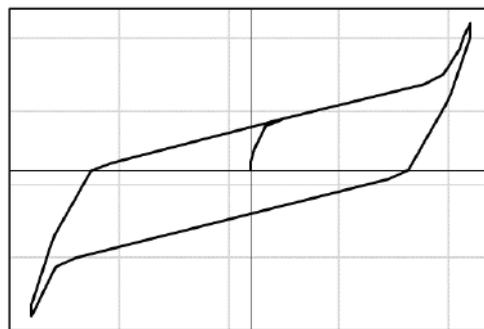
Fig. 3. Backbone curve and hysteresis loop of QTFP isolator
