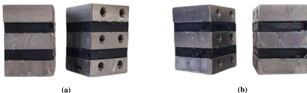
Fig. 3. Damper units of various rubber pads: a) Ref. CIIR pads; and b) Mod. CIIR pads
