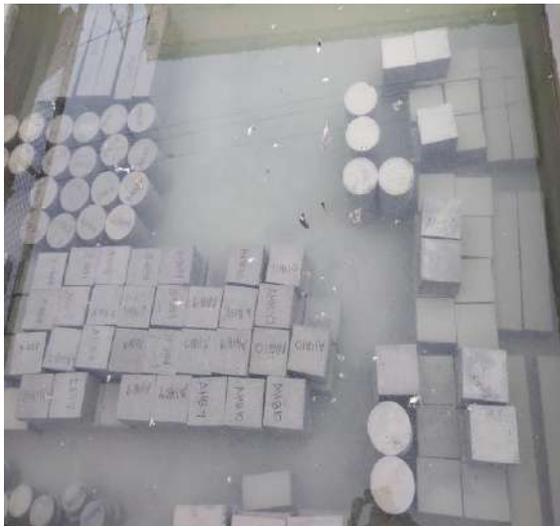
**Fig. 4.** Curing of specimens in curing tank
