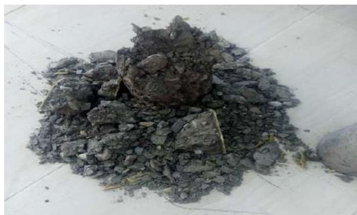
Fig. 10. View of a cylinder tested in compression (GE = 0.66%)
