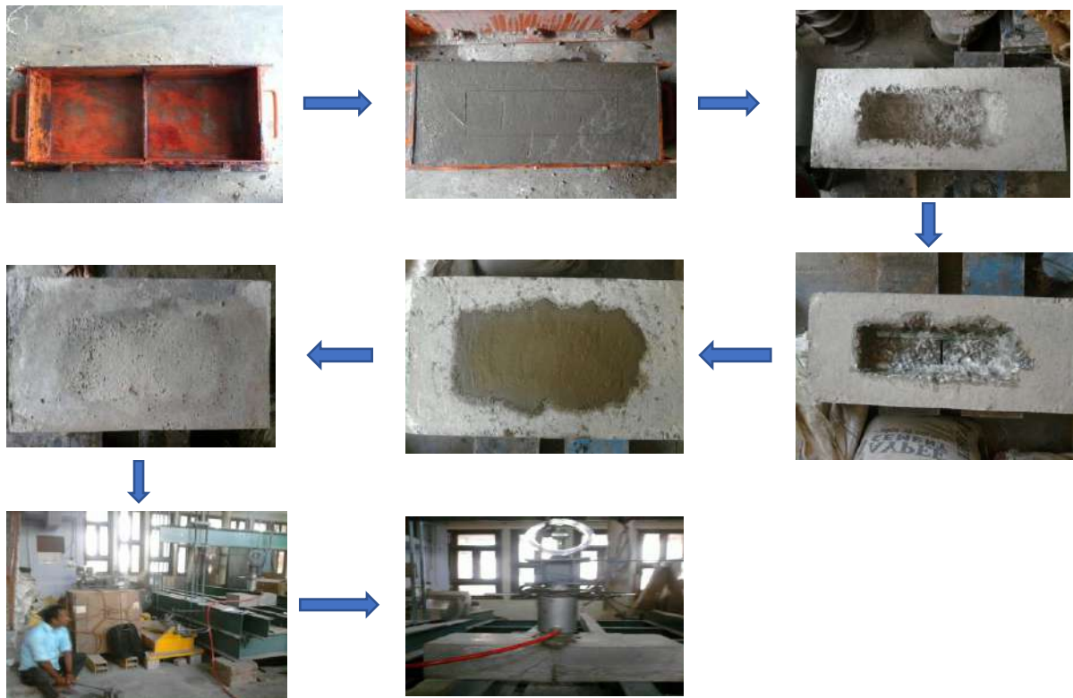
Fig. 9. Schematic representation of rehabilitation and testing of pavement prototypes
