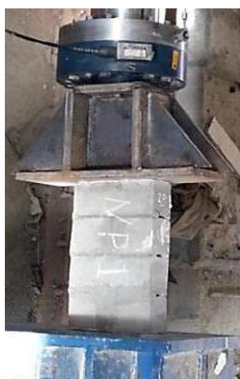
Fig. 6. An overview of the compression test setup for the masonry prisms
