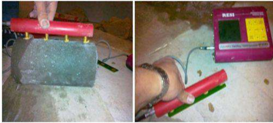
Fig. 5. Measuring device electrical resistivity
