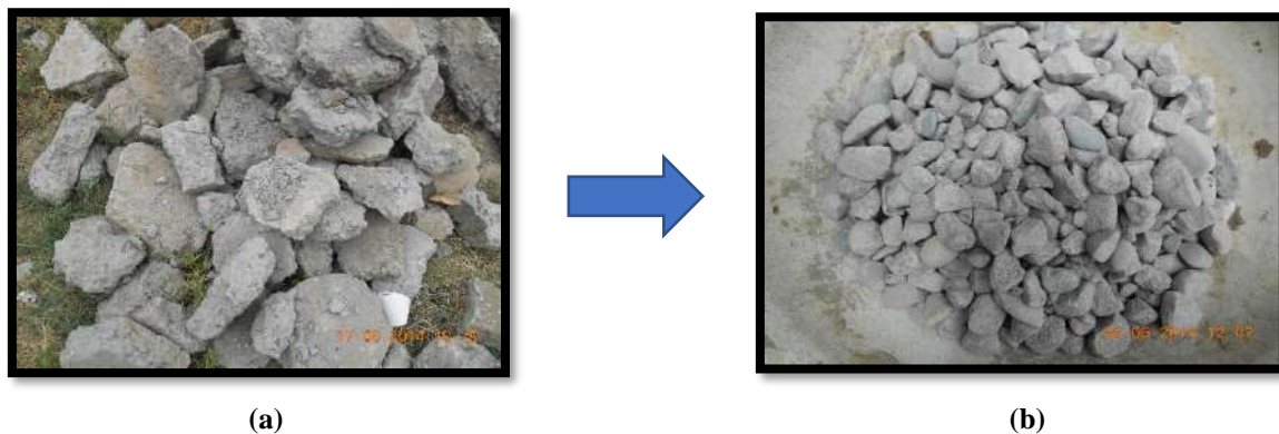
Fig. 1. a and b) Recycled concrete aggregates processed from demolished concrete waste
