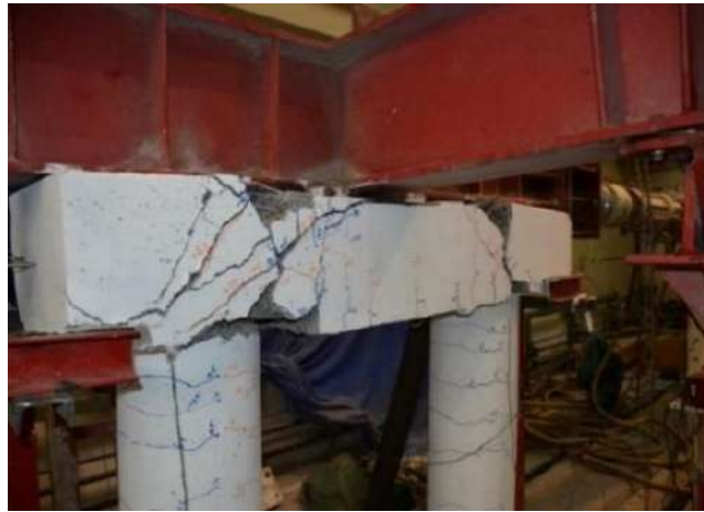
Fig. 14. Ultimate damage mechanism for SP-80
