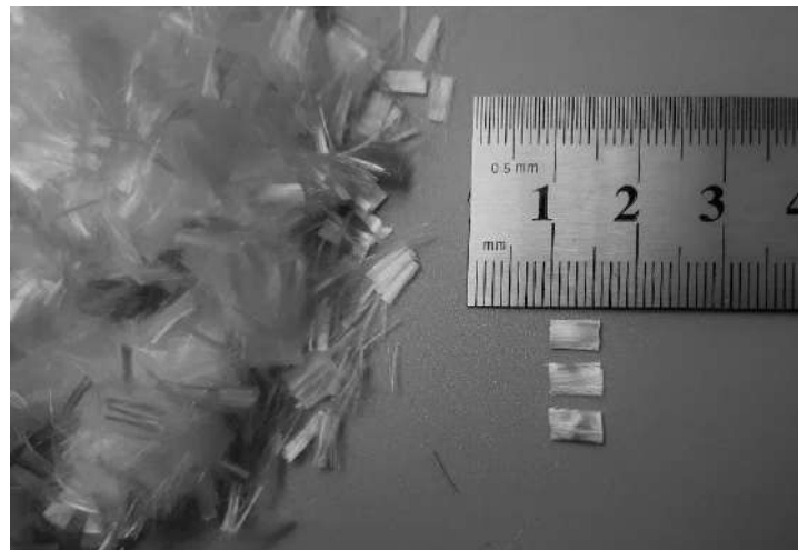
Fig. 3. Polyvinyl alcohol fiber with a length of 6 mm
