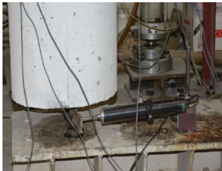
Fig. 4. Connecting the specimen to a steel beam (rigid floor)
