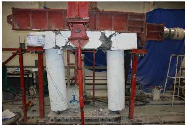
Fig. 15. Ultimate damage mechanism for SP-90
