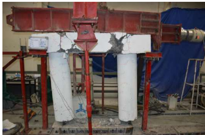
Fig. 30. Failure mode of SP-90
