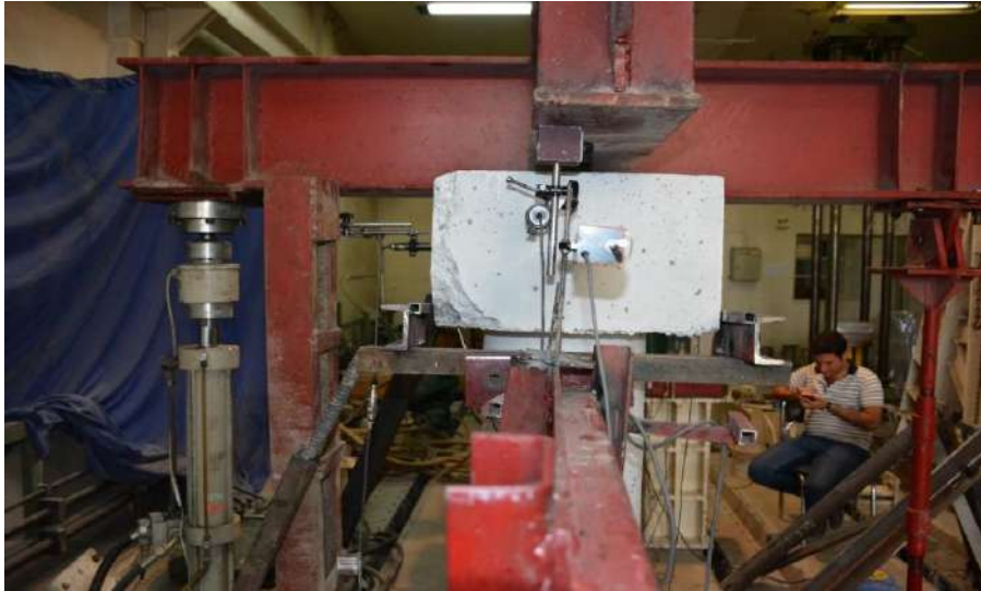
Fig. 8. Applying gravity load
