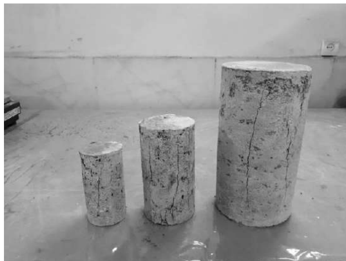
Fig. 4. Typical crack pattern of failed cylindrical specimens
