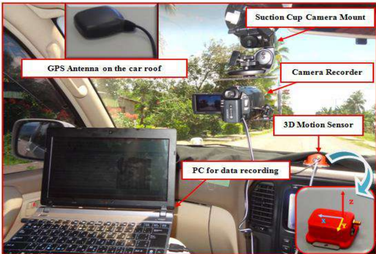
Fig. 1. Arrangement of measuring equipment installed in a car
