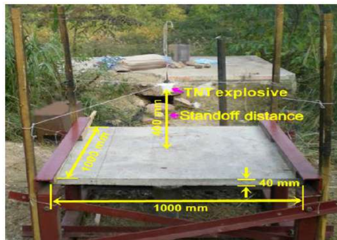
Fig. 6. Laboratory specimen of reinforced concrete slab in reference (Wang et al., 2013)
