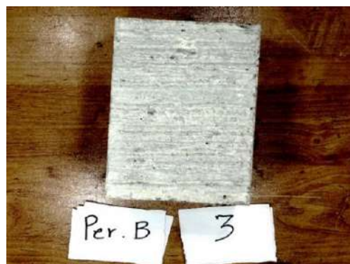
Fig. 17. A specimen with perpendicular brushing texture on it
