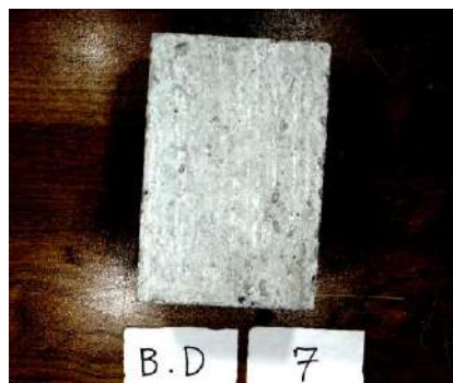
Fig. 19. Specimen with burlap dragging on it
