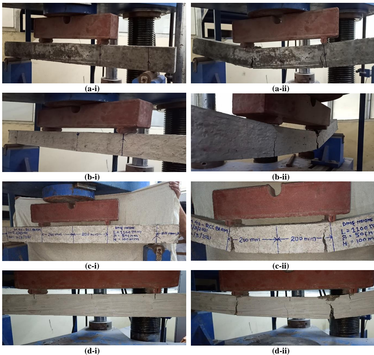
Fig. 7. Reinforced concrete beam of: a) M20; b) M30; c) M40; and d) M50 concrete grades; i) Before; and ii) After the four-point bending test
