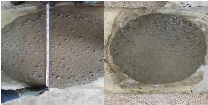
Fig. 3. SCC slump-flow test
