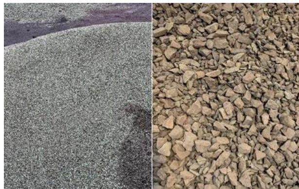
Fig. 2. Ferro-silicomanganese slag of ferroalloy industries
