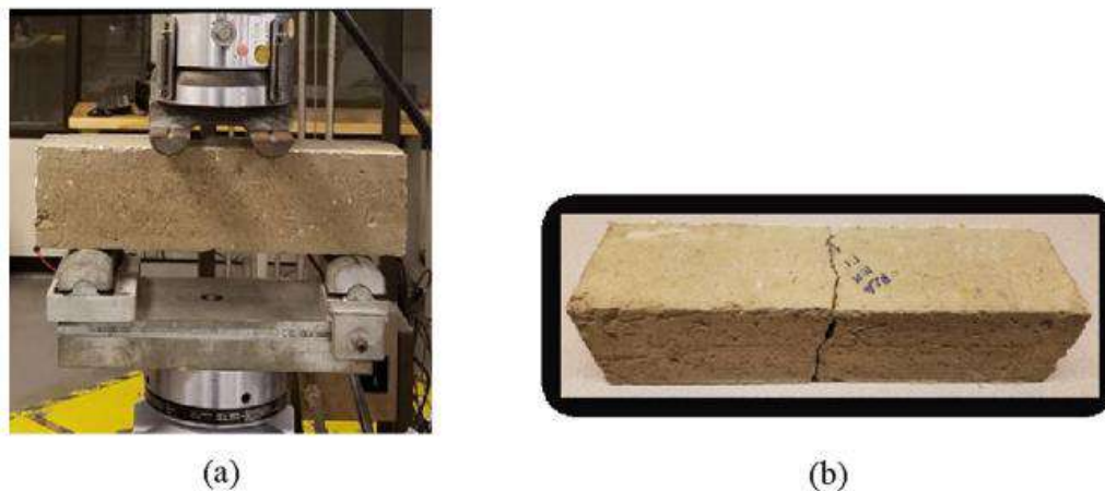
Figure 12. (a) Flexure strength test (b) Failed specimen
