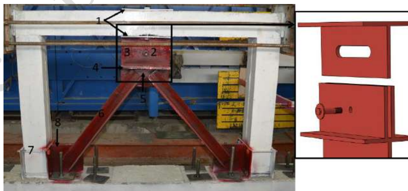
1-PL300x150x10 mm 2-Bolt16mm Gr8.8 3-3PL300x150x10 mm 4-3PL300x150x15 mm 5-PL300x120x10 mm 6-2L80x8 mm 7-4Bolt 14mm Gr8.8 8-PL200x200x10 mm
