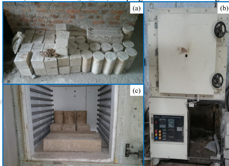
Fig. 2. Photographs of Experimental programs (a) casted samples (b) Muffle furnace (c) Samples in muffle furnace
