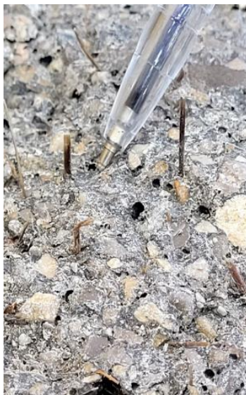
Fig. 7. The failure of the cube specimen with the compressive strength device, and the specimen broken with palm fibers
