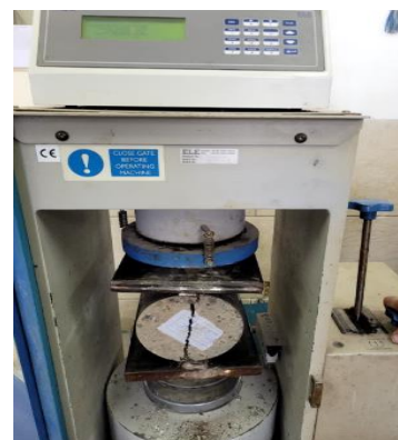
Fig. 8. Failure of the cylindrical test piece with the Brazilian device and the test piece broken with palm fibers
