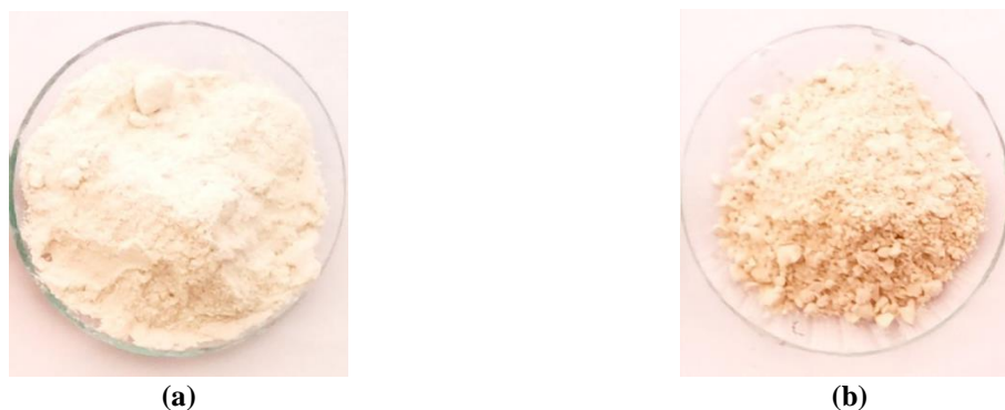
Fig. 1. Samples of raw clays before the calcination process (Bahman-Zadeh et al., 2022): a) Clay Sample 1 (kaolinite content: 19.4%); and b) Clay Sample 2 (kaolinite content: 28.7%)
