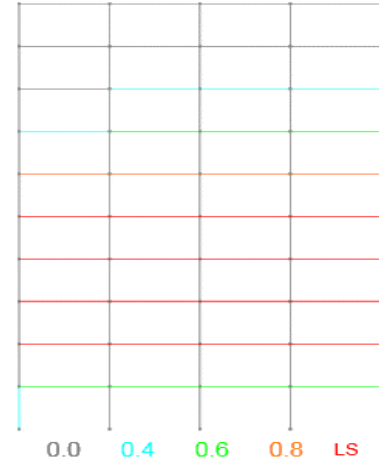
Fig. 9. Structural performance of the ten-story building under loma record with 0.7 g maximum acceleration
