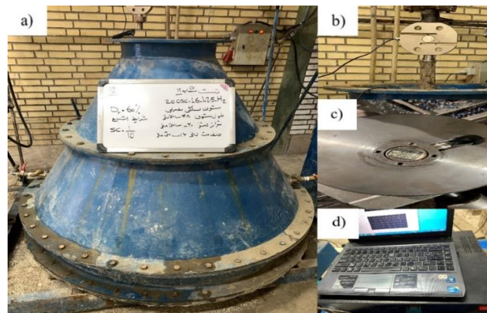
Fig. 3. Overview of FCV apparatus and FCV accessories: a) FCV; b) Load cell; c) Mini-load cell, loading plate; and d) Data logger and laptop
