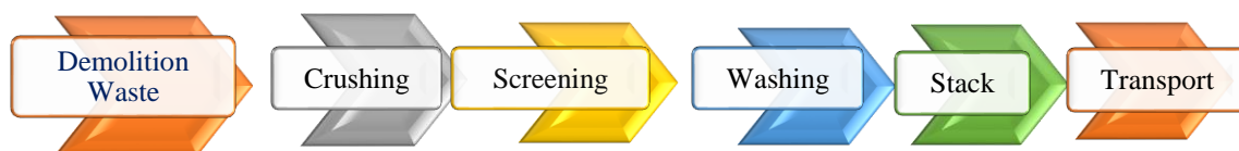
Fig. 2. Process for production of recycled concrete aggregate
