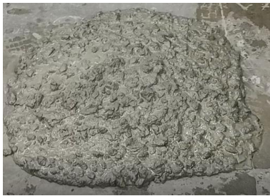
Fig. 6. Slump flow test on self-compacted recycled aggregate concrete
