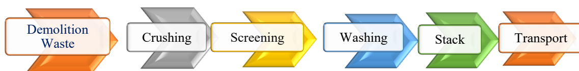
Fig. 2. Process for production of recycled concrete aggregate
