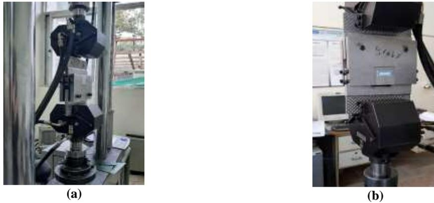
**Fig. 8.** Cyclic shear test setup: a) Installation of damper specimen in test machine; and b) Front view of damper under cyclic loading
