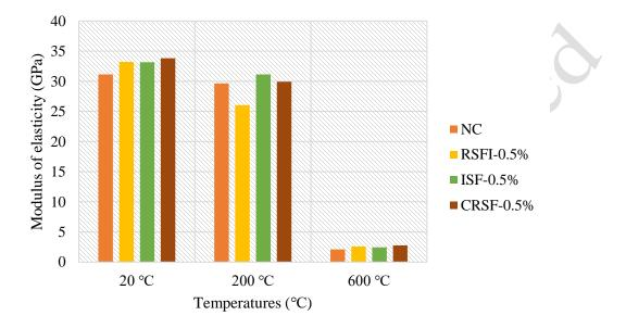
Fig. 11 The secant modulus of elasticity of the specimens at different temperatures
