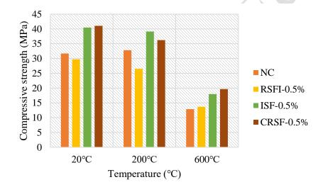
Fig. 9 Compressive strengths of specimens at different temperatures
