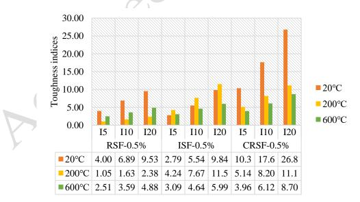
Fig. 17 Toughness indices at different temperatures
