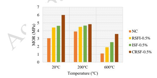
Fig. 16 MOR of specimens at different temperatures
