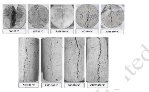
Fig. 12 Tensile failure mode of specimens at different temperatures
