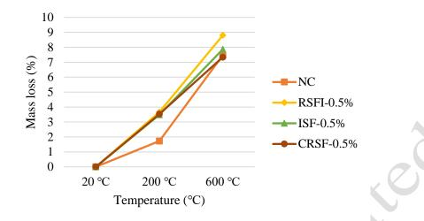
Fig. 7 Mass loss of specimens at different temperatures
