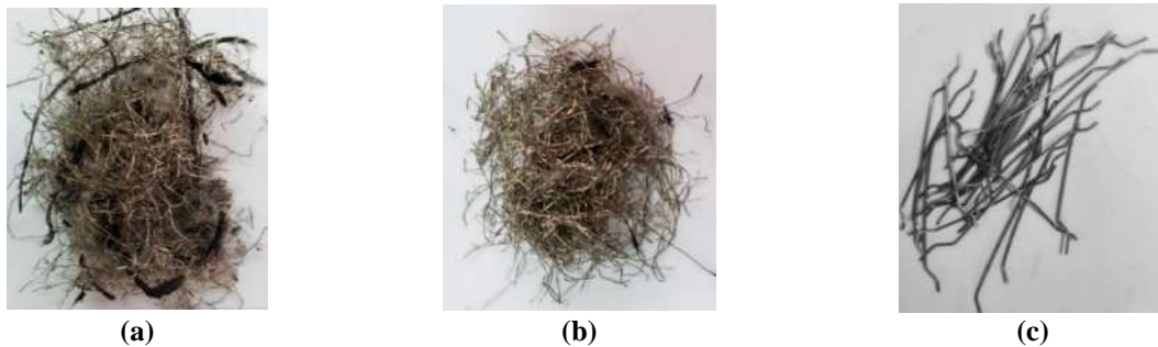
Fig. 1. Steel fibers used: a) RSFI; b) CRSF; and c) ISF
