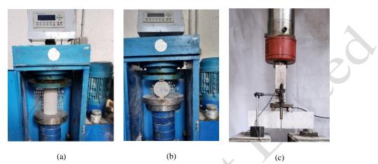
Fig. 4 Setup for: (a) compressive, (b) tensile, and (c) flexural test
