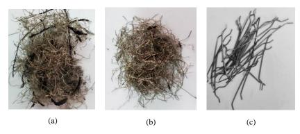
Fig. 1 Steel fibers used: (a) RSFI, (b) CRSF, and (c) ISF
