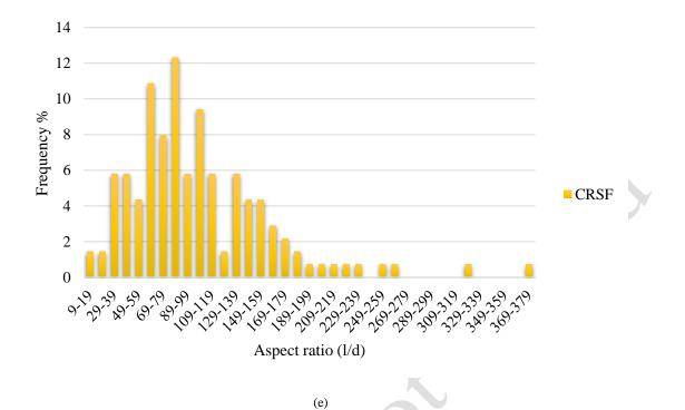
Fig. 2 Geometric analysis of recycled steel fibers: (a) diameter of RSFI and CRSF, (b) length of RSFI, (c) aspect ratio of RSFI, (d) length of CRSF, and (e) aspect ratio of CRSF
