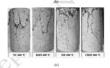
Fig. 8 Compressive failure mode of specimens: (a) Ambient temperature, (b) 200 °C, (c) 600 °C
