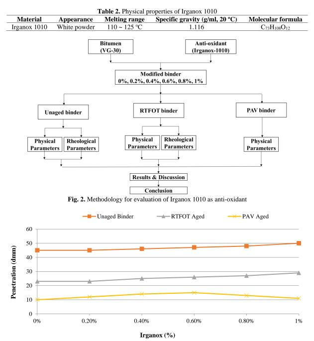
Fig. 3. Effect of Irganox 1010 on penetration values of unaged, RTFO aged and PAV aged binders
