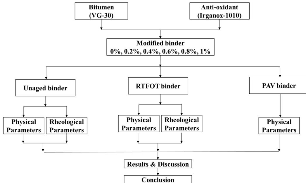
**Fig. 2.** Methodology for evaluation of Irganox 1010 as anti-oxidant
