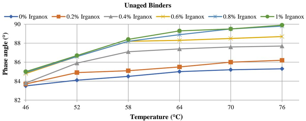
Fig. 9. Phase angle variation of unaged binders
