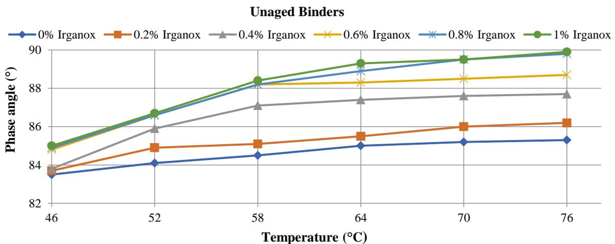
Fig. 9. Phase angle variation of unaged binders
