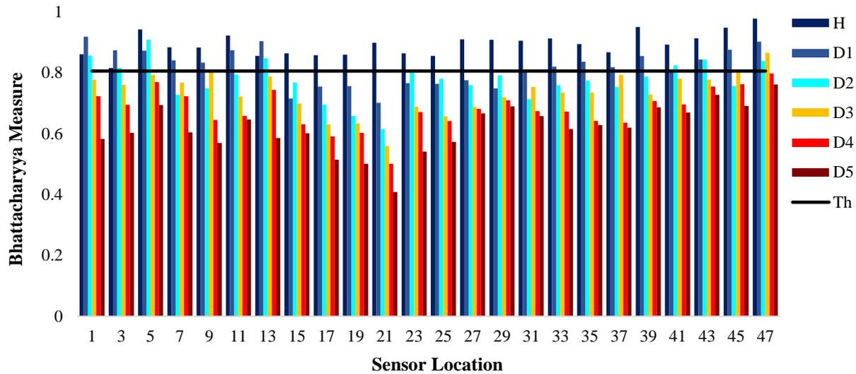
**Fig. 4.** The Bhattacharyya measure of odd DOFs of beam structure in different structural states
