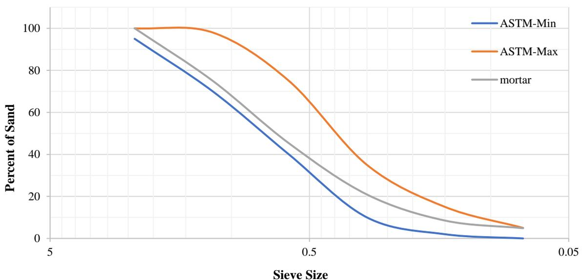
**Fig. 4.** Sand-grading for the (full-scale) mortar/grout**Table 5.** Compressive strength of full-scale mortar specimens
