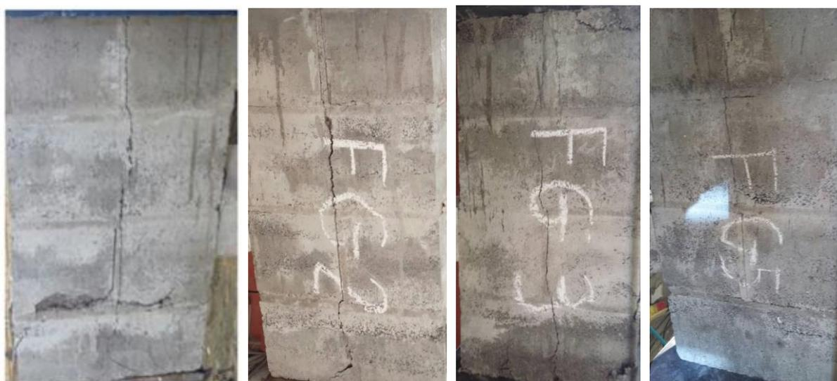
(a) Typical failure modes in the FG
