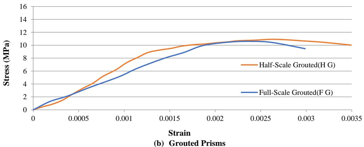
**Fig. 7.** Stress-strain curves of full-scale and half-scale masonry prisms
