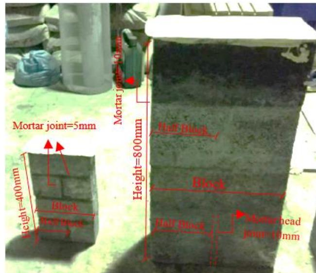
**Fig. 5.** Typical half-scale and full-scale masonry prisms
