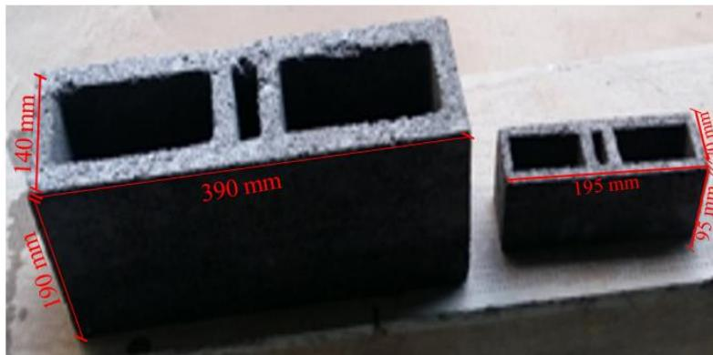
Fig. 1. Typical concrete masonry unit (full-scale and half-scale)
