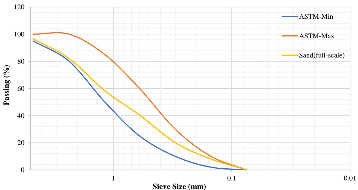
Fig. 2. Grading of aggregates for the full-scale blocks
