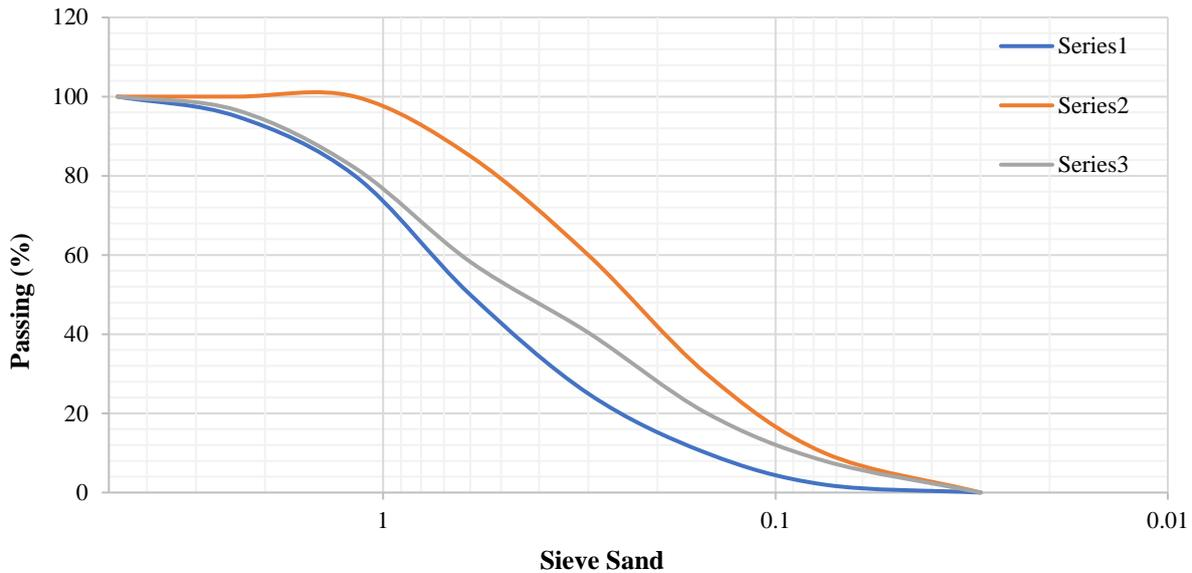
Fig. 3. Grading of aggregates for the half-scale blocks
