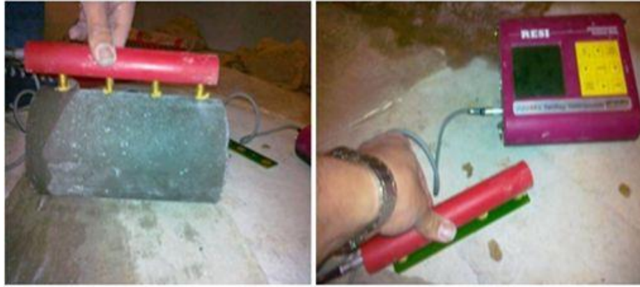
Fig. 5. Measuring device electrical resistivity
