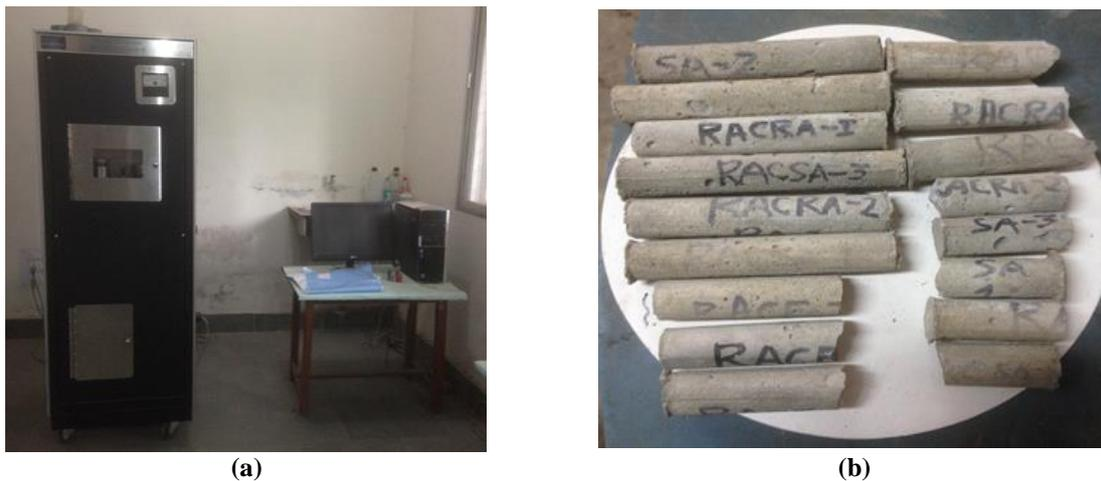
**Fig. 6.** a) Mercury Porosimeter; and b) Concrete specimens
