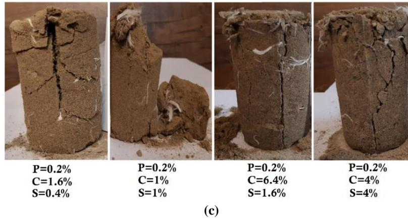
**Fig. 13.** Failure patterns of the: a) Specimens treated with steel slag and fiber mixture; b) Specimens treated with cement and fiber mixture; and c) Specimens treated with cement, steel slag and fiber mixture
