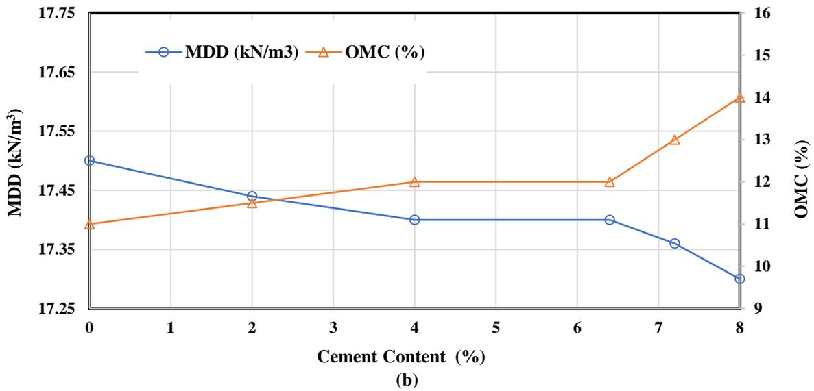
Fig. 2. Variation of OMC and MDD of specimens treated with cement and steel slag: a) Additive content of 2%; and b) Additive content of 8%
