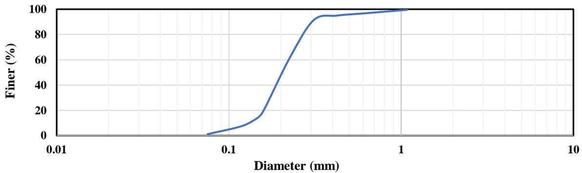
Fig. 1. Grain-size distribution curve of Varzaneh sand
