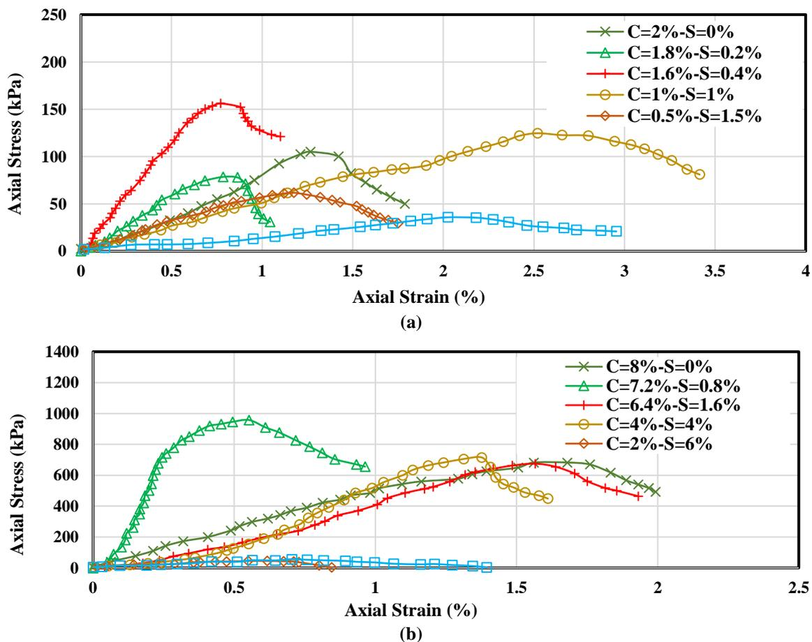
Fig. 4. Stress-strain curves of the specimens treated with cement and steel slag mixture: a) Additives content of 2%; and b) Additives content of 8%
