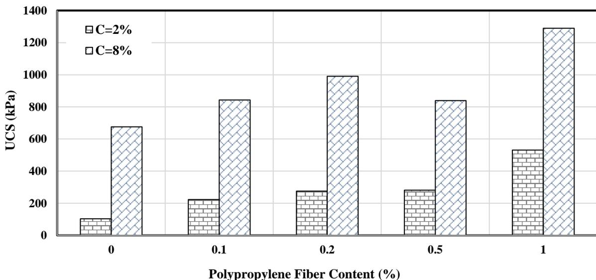
**Fig. 7.** UCS values of the fiber-reinforced cement-stabilized specimens
