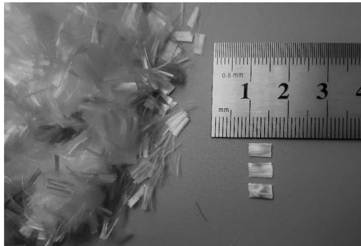
Fig. 3. Polyvinyl alcohol fiber with a length of 6 mm
