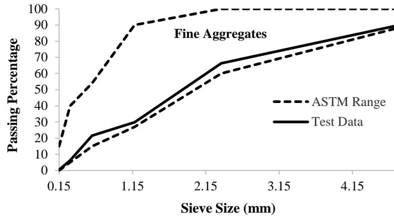
Fig. 1. Gradation of the utilized fine aggregates
