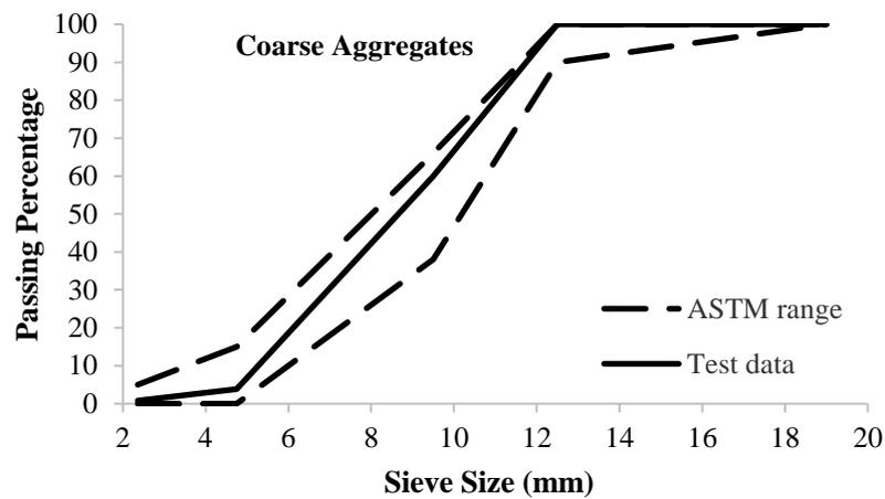
Fig. 2. Gradation of the utilized coarse aggregates
