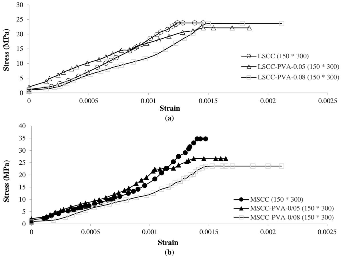
**Fig. 9.** a) Pre-peak stress-strain curve of low strength cylinders with the diameter of 150 mm containing different dosages of PVA fibers; and b) Pre-peak stress-strain curve of medium strength cylinders with the diameter of 150 mm containing different dosages of PVA fibers
