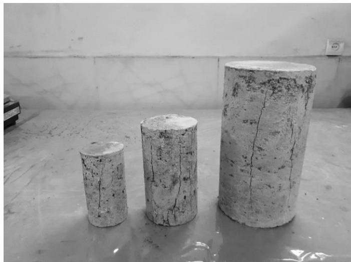
**Fig. 4.** Typical crack pattern of failed cylindrical specimens
