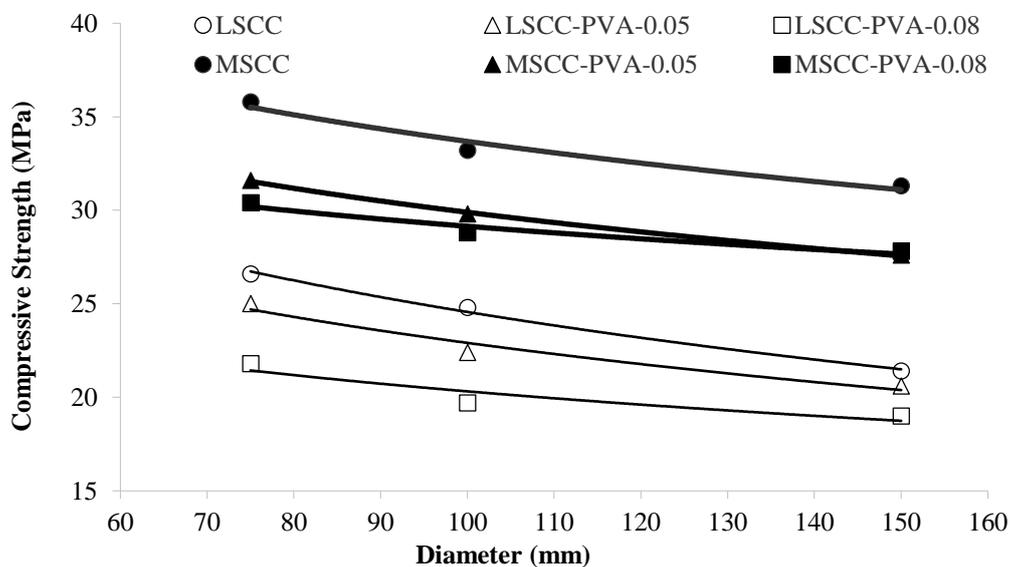
**Fig. 5.** Compressive strength reduction of low strength and medium strength cylindrical specimens with different diameters
