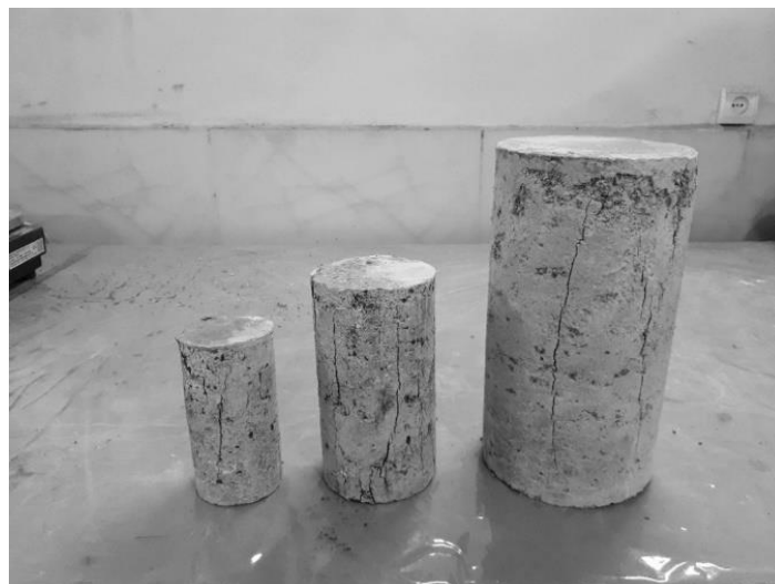
Fig. 4. Typical crack pattern of failed cylindrical specimens
