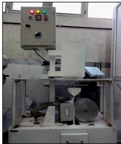
Fig. 2. The employed abrasion machine
