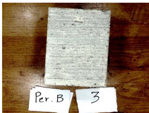
Fig. 17. A specimen with perpendicular brushing texture on it
