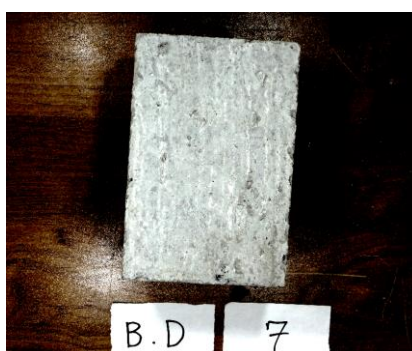
Fig. 19. Specimen with burlap dragging on it
