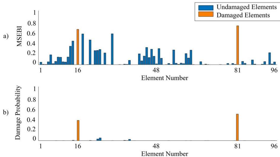
**Fig. 9.** Damage case D6 considering modes 1 to 5: a) MSEBI values; and b) Dempster-Shafer theory damage probabilities
