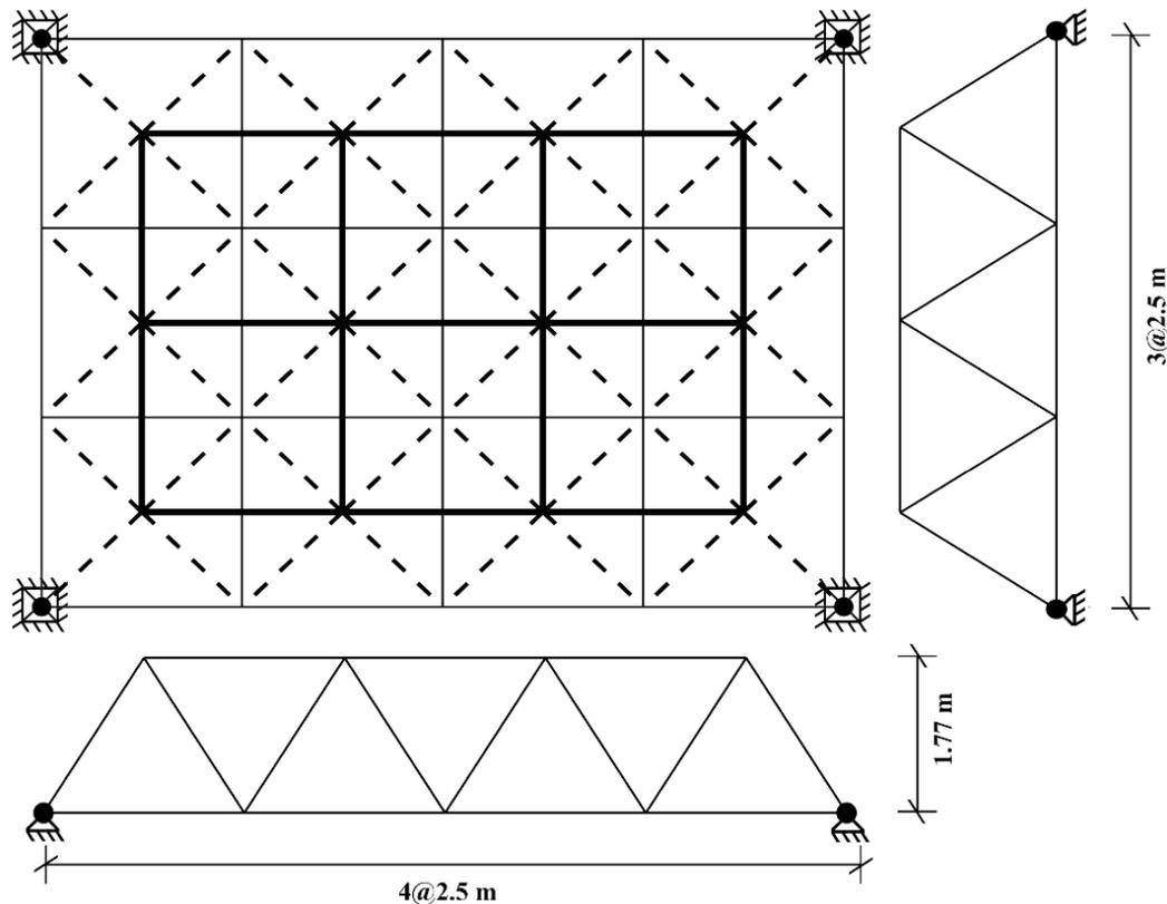
Fig. 1. Double layer grid chosen for study
