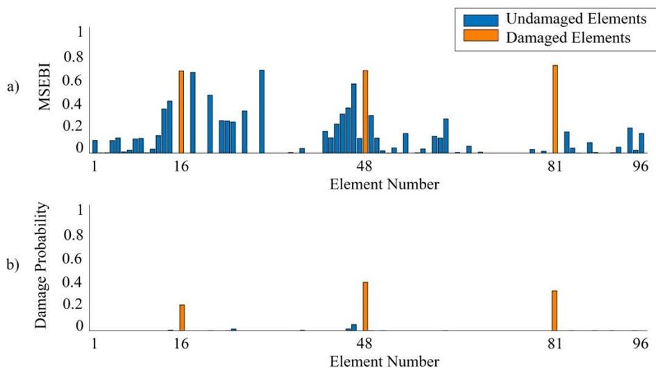
**Fig. 10.** Damage case D7 considering modes 1 to 5: a) MSEBI values; and b) Dempster-Shafer theory damage probabilities
