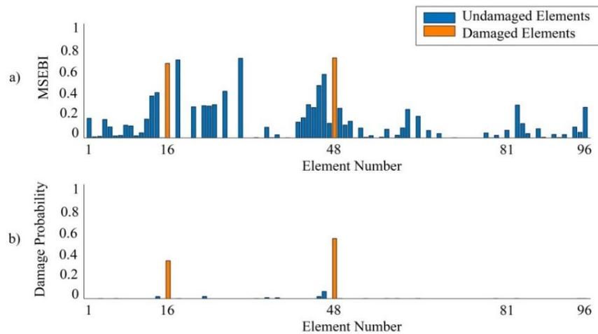
**Fig. 7.** Damage case D4 considering modes 1 to 5: a) MSEBI values; and b) Dempster-Shafer theory damage probabilities
