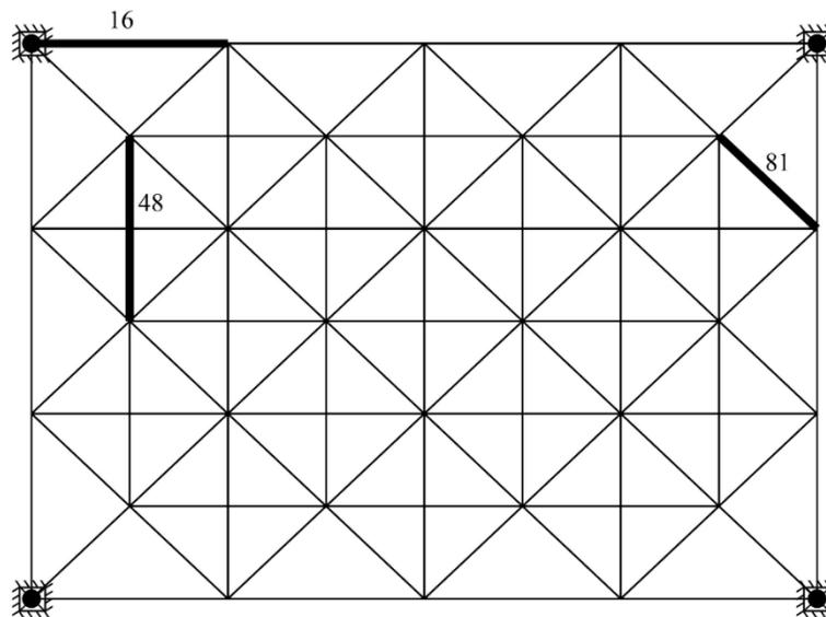
Fig. 2. Damaged elements
