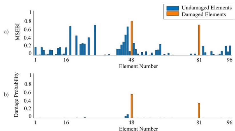
**Fig. 8.** Damage case D5 considering modes 1 to 5: a) MSEBI values; and b) Dempster-Shafer theory damage probabilities
