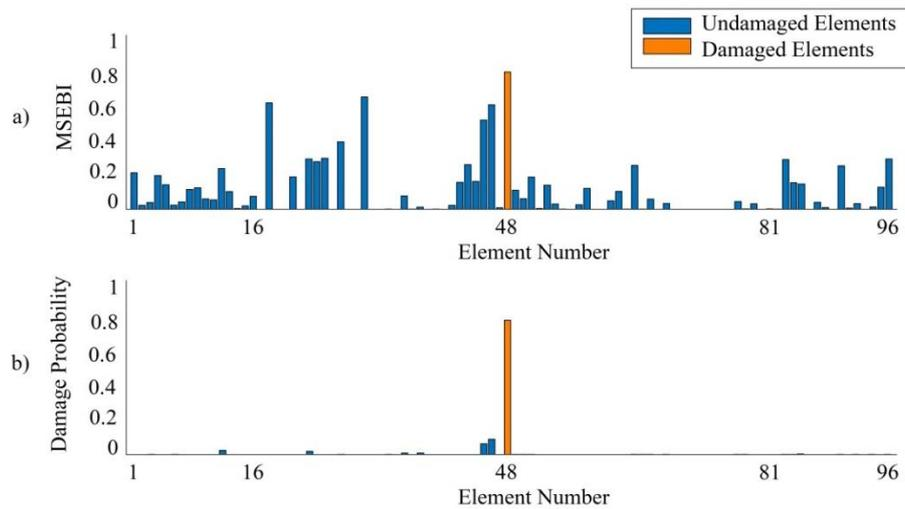
**Fig. 5.** Damage case D2 considering modes 1 to 5: a) MSEBI values; and b) Dempster-Shafer theory damage probabilities
