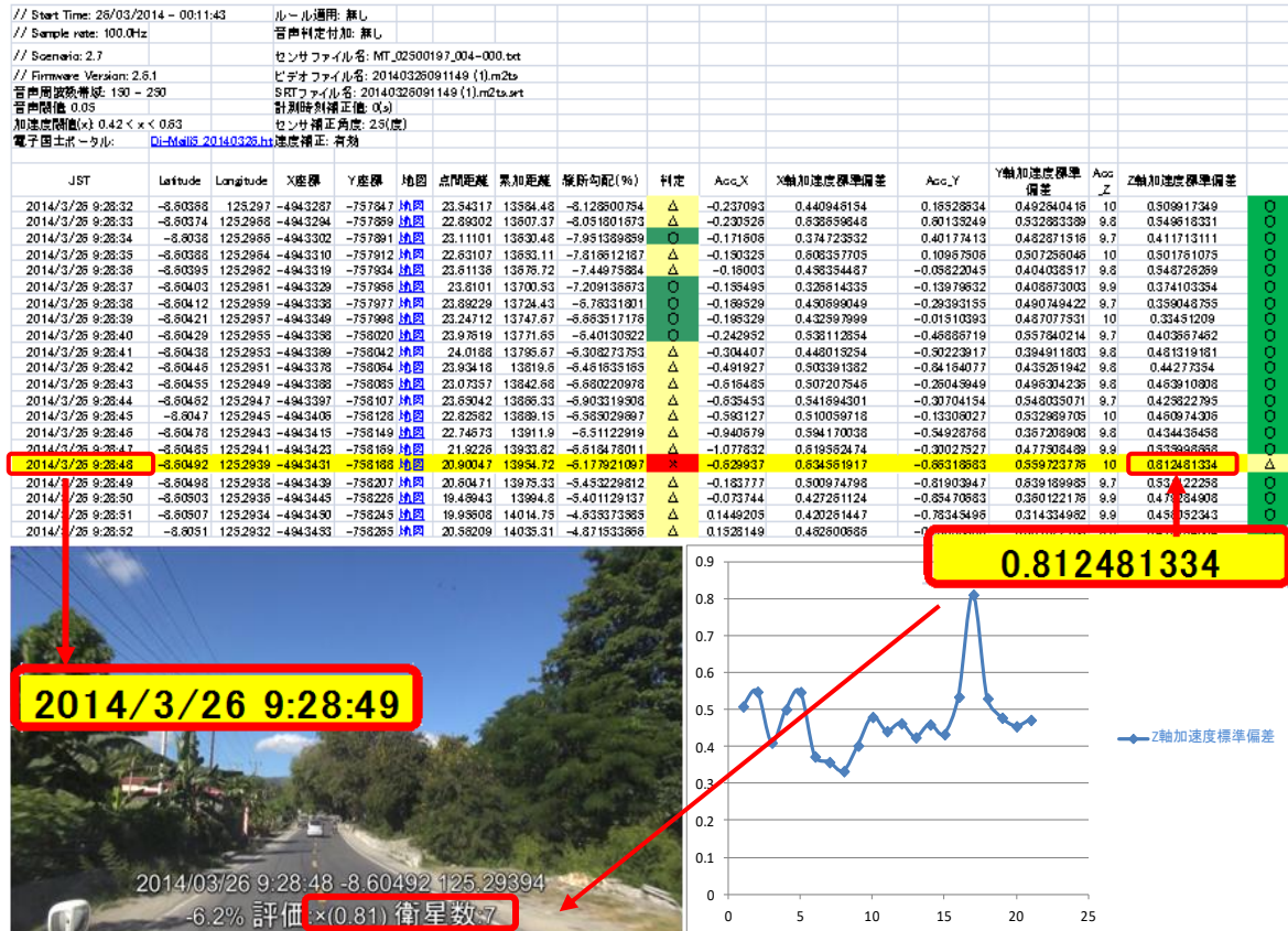
Fig. 14. Evaluation result for GOOD Timor-Leste road, obtained using Ippo-Campo
