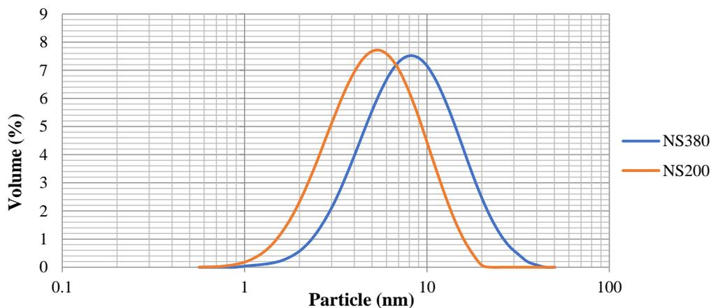
Fig. 2. Gradation of the nano particles used in this research
