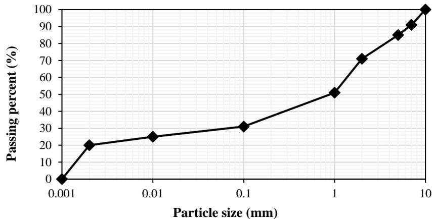
Fig. 1. Gradation curve of the soil used in this research
