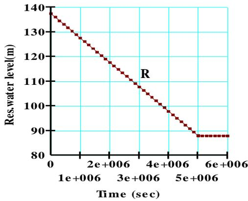
Fig. 12. Drawdown rate (head versus time), GeoStudio
