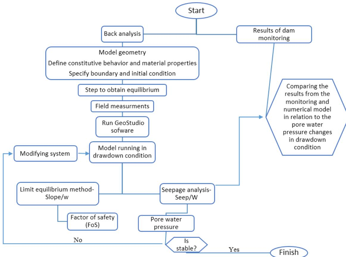
Fig. 9. Back analysis method and solution algorithm
