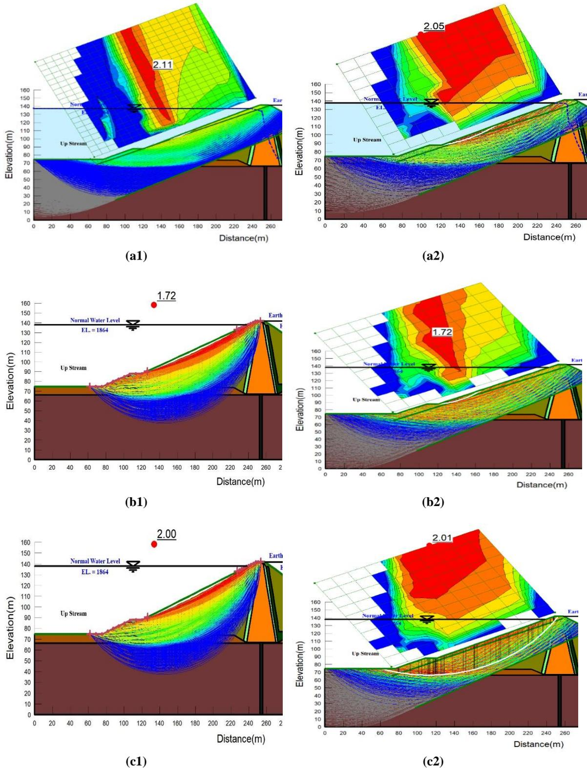
**Fig. 18.** Critical slope surface and factor of safety after rapid drawdown: a) Before drawdown; b) After 42 day; c) After 58 day (1: Morgenstern-Price; and 2: Bishop)
