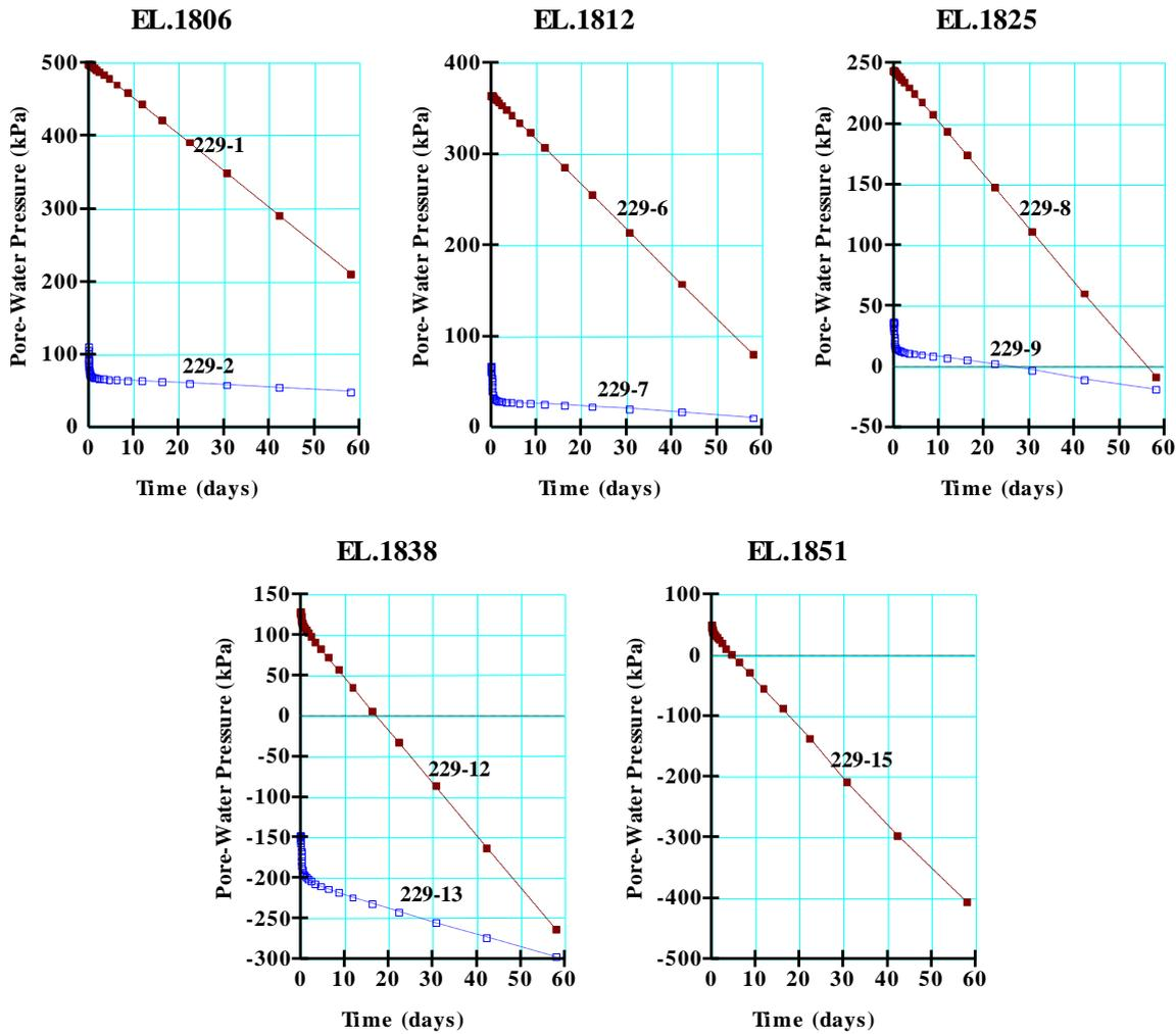
Fig. 15. Pore water pressure in the core of Eyvashan earth dam during rapid drawdown (GeoStudio)
