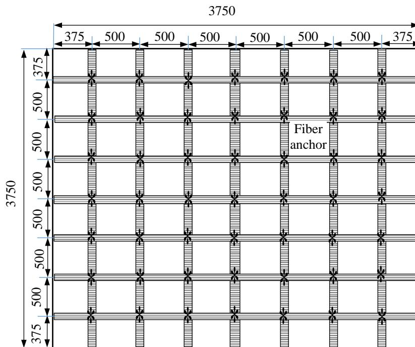
**Fig. 11.** Plan view of flat plate strengthened with GFRP (Qian et al., 2014)
