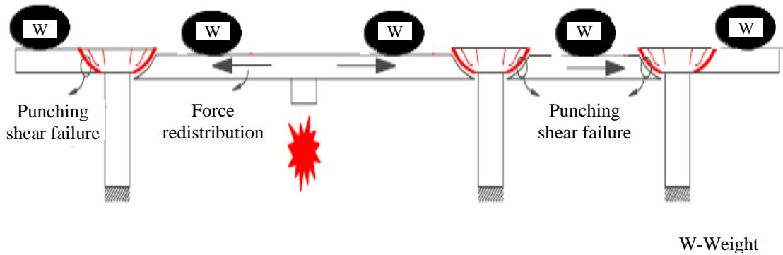
**Fig. 1.** Propagation of punching shear failure (Mitchell et al., 1984)
