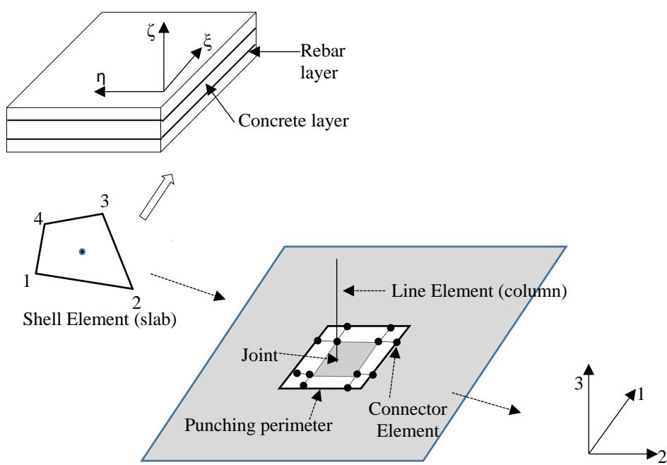
**Fig. 9.** Schematic sketch macro model for flat plate
