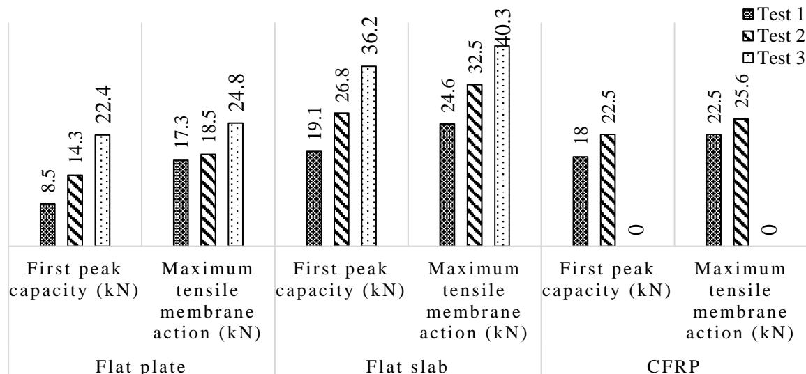
**Fig. 12.** Comparison of different parameter values**Table 5.** Reinforcement details
