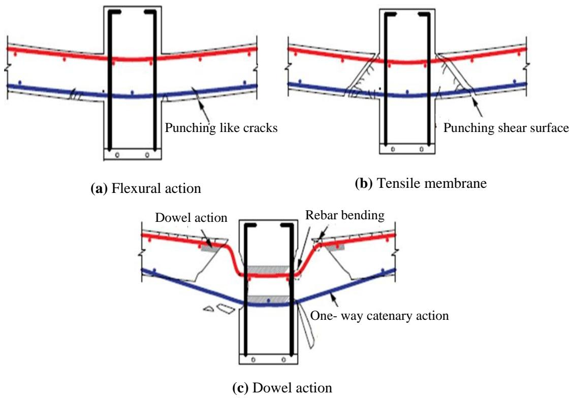
**Fig. 5.** Failure modes (Xue et al., 2018)
