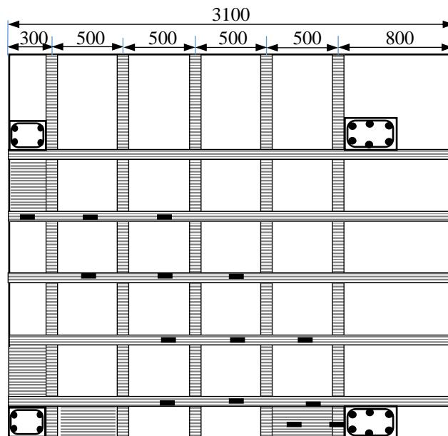
**Fig. 10.** Plan view flat plate strengthened with CFRP (Qian et al., 2013)
