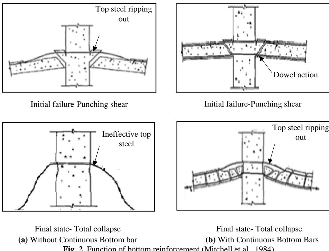
**Fig. 2.** Function of bottom reinforcement (Mitchell et al., 1984)
