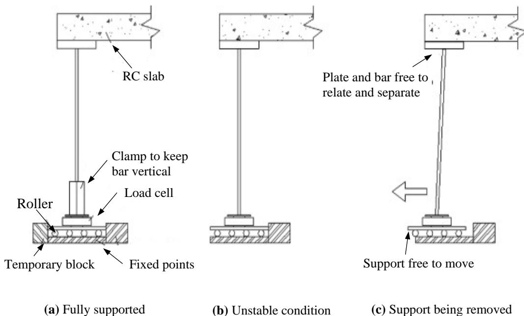
**Fig. 7.** The mechanism of the loss of the column (Russel et al., 2015)
