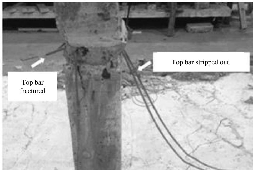
**Fig. 8.** Post punching shear failure pattern (Peng et al., 2017)
