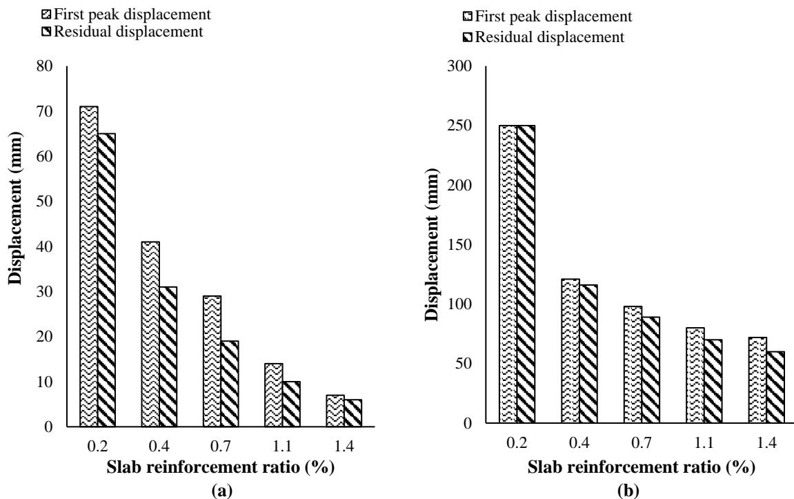
**Fig. 6.** Effect of reinforcement ratio: a) Flat slab structure and; b) Flat plate structure
