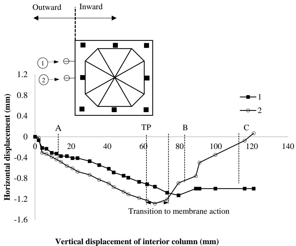
**Fig. 4.** Relationship between horizontal and vertical displacement (Yi et al., 2014)
