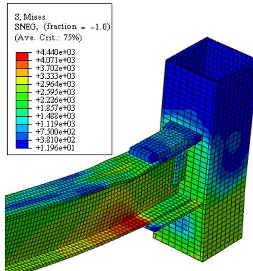
(c) Stress distribution for corner column without transverse beam at 43 cm vertical displacement
