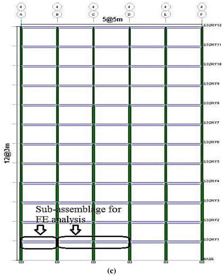
Fig. 2. Structural configuration of the models chosen: a) Structures plan; b) Seven story frame and; c) Twelve story frame
