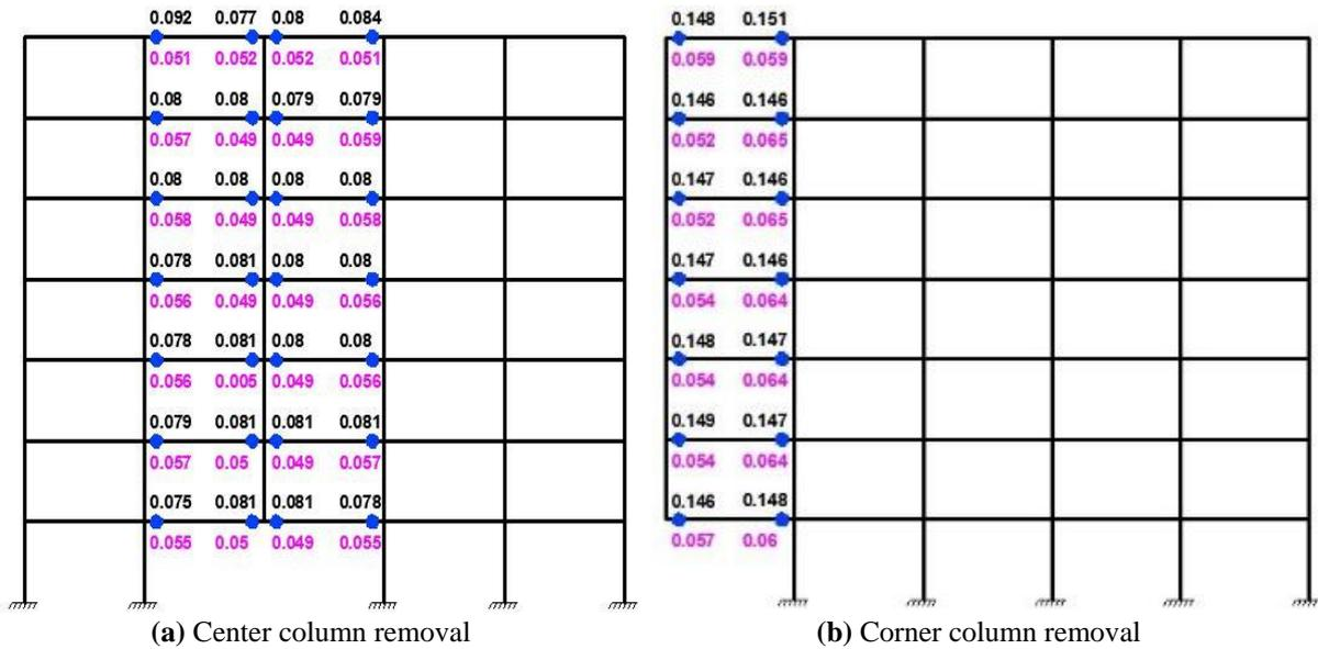
Fig. 7. Rotation of beams (in radian) for seven story building with and without considering out of plane effect with DoD loading
