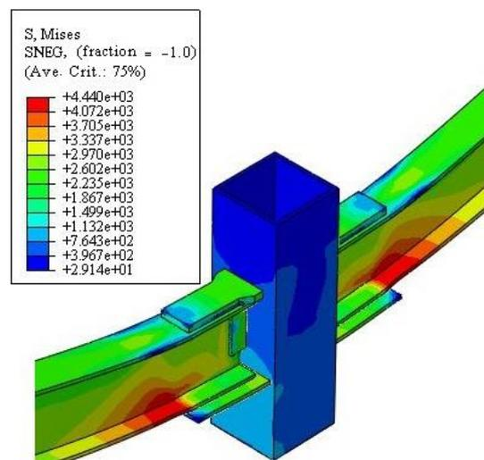
(b) Stress distribution for middle column without transverse beam 51 cm vertical displacement
