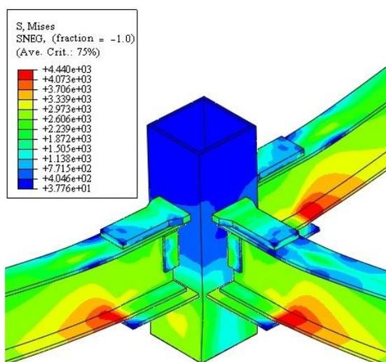
(a) Stress distribution for middle column with transverse beam at 61 cm vertical displacement
