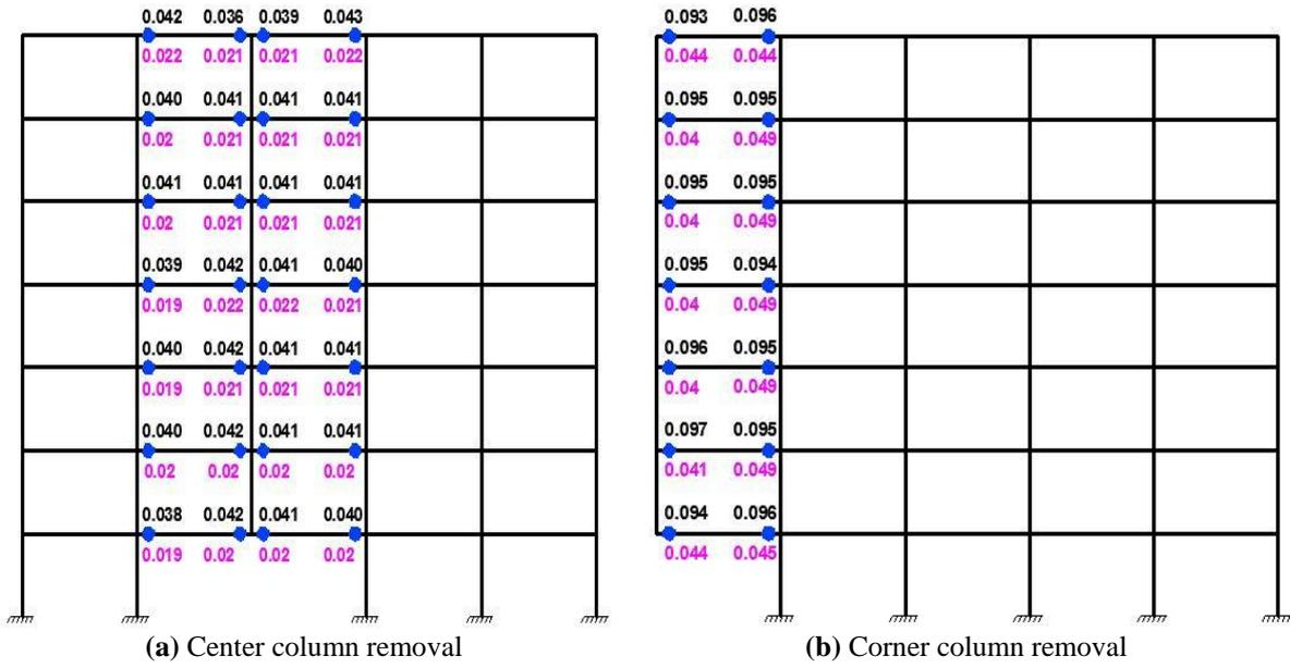
Fig. 6. Rotation of beams (in radian) for seven story building with and without considering out of plane effect with GSA loading
