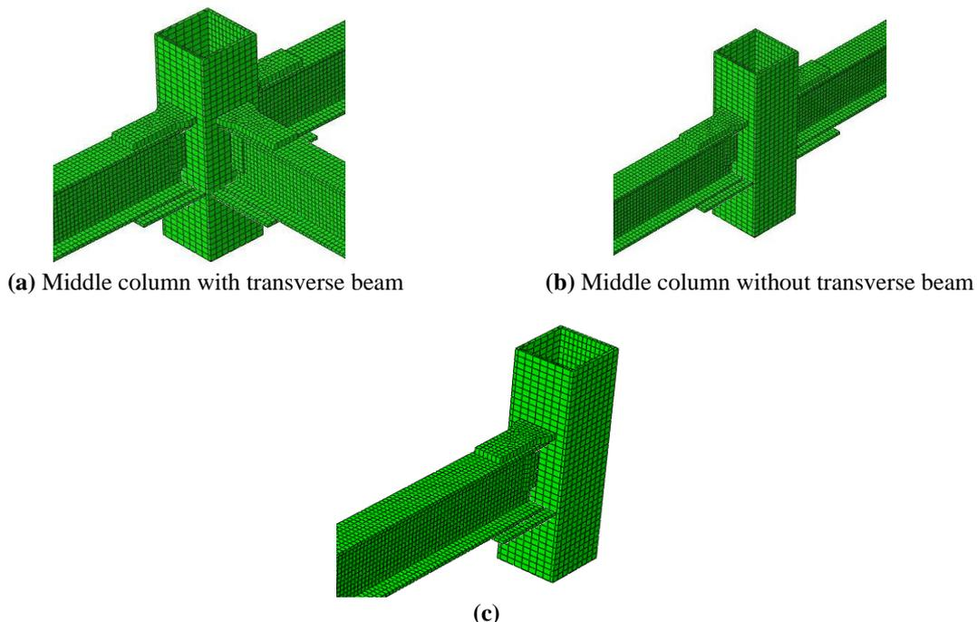
**Fig. 11.** Finite Element model of seven story building in two different conditions
