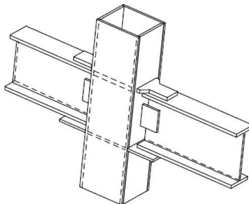
**Fig. 8.** Welded flange plate connection
