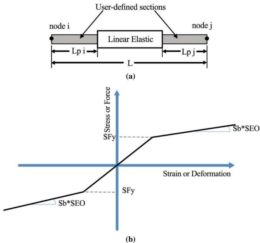
Fig. 3. Opensees element and material: a) Beam with hinge element and; b) Steel01 material model
