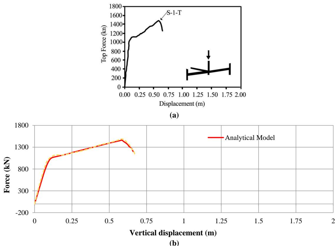
**Fig. 10.** First story Force-Displacement relation for non RBS connections without transverse beam: a) Khandelwal and El-Tawil (2007) and; b) Present analysis
