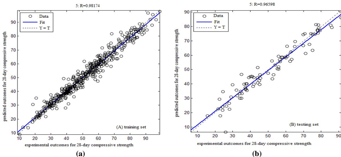
**Fig. 5.** Predicted outcomes vs. experimental outcomes for 28-day compressive strength: a) Training set and; b) Testing set
