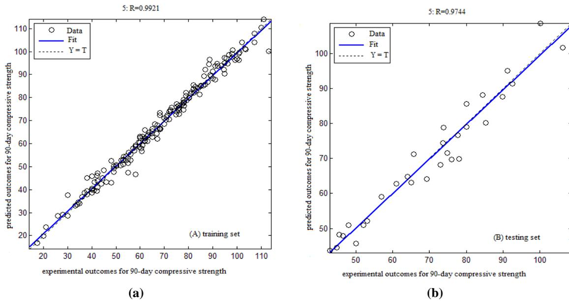
Fig. 6. Predicted outcomes vs. experimental outcomes for 90-day compressive strength: a) Training set; b) Testing set
