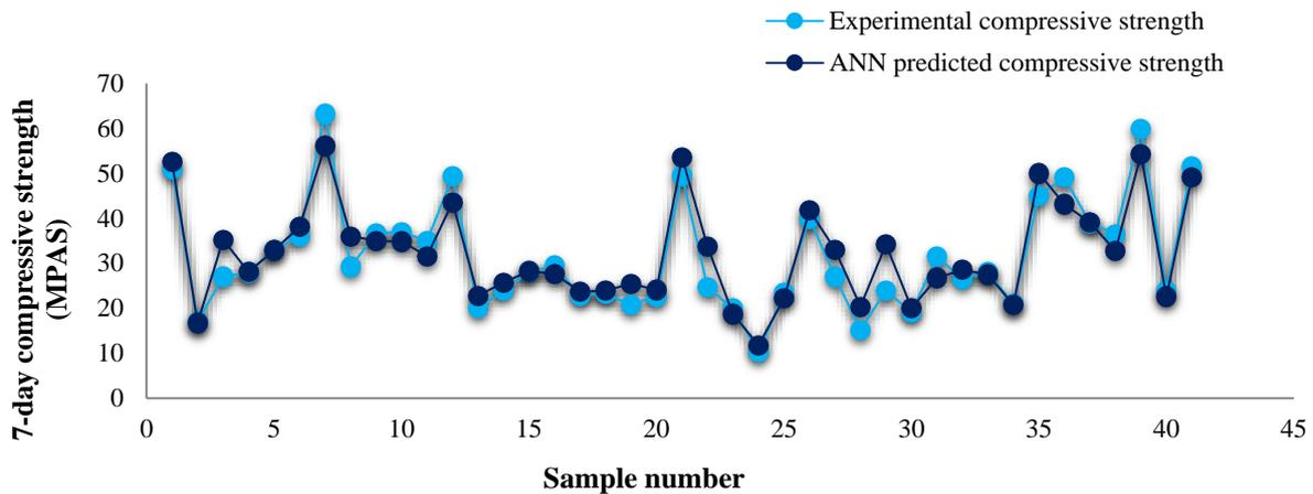
Fig. 8. Comparison between the predicted and experimental values of 7-day compressive strength
