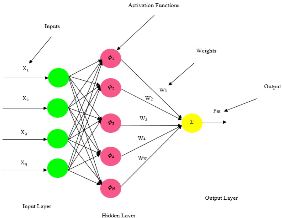
**Fig. 3.** Architecture of RBF neural network
