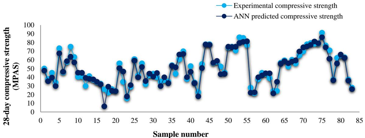
Fig. 9. Comparison between the predicted and experimental values of 28-day compressive strength
