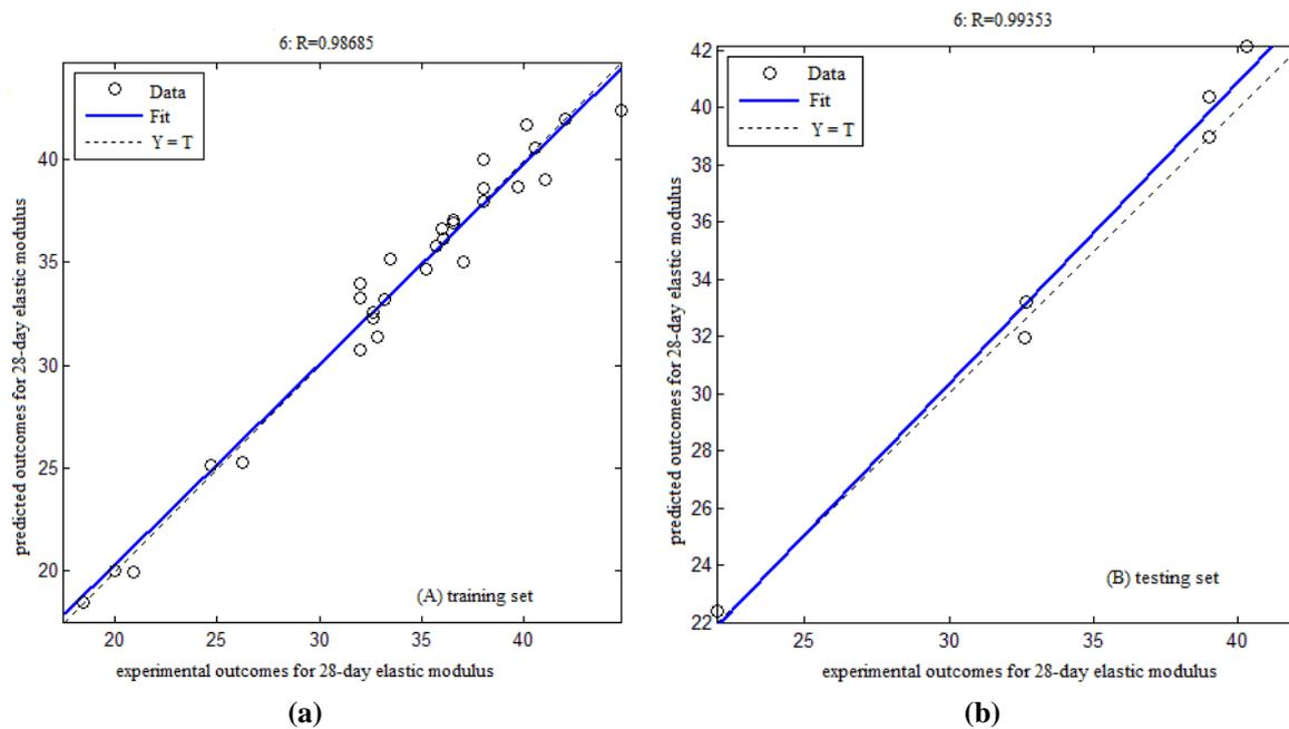
Fig. 7. Predicted outcomes vs. experimental outcomes for 28-day elastic modulus: a) Training set and; b) Testing set
