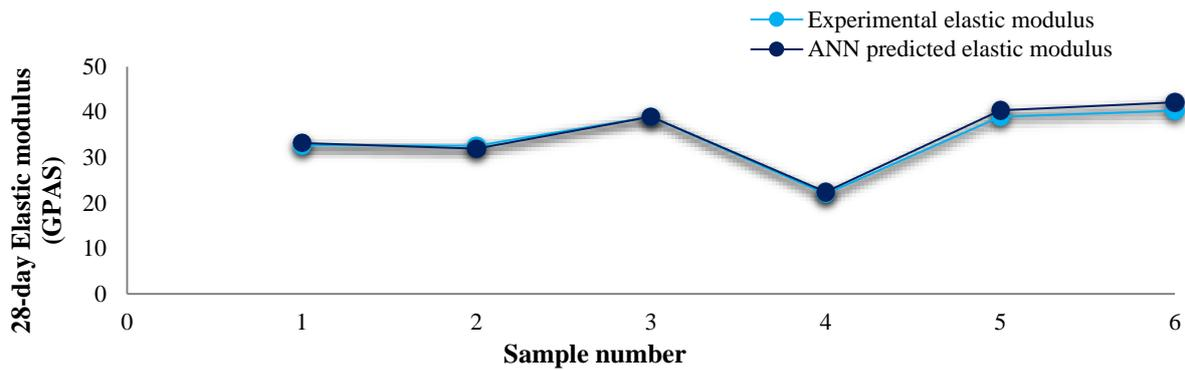
Fig. 11. Comparison between the predicted and experimental values of 28-day elastic modulus
