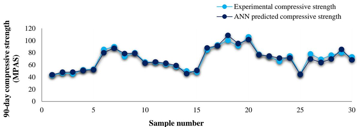
Fig. 10. Comparison between the predicted and experimental values of 90-day compressive strength
