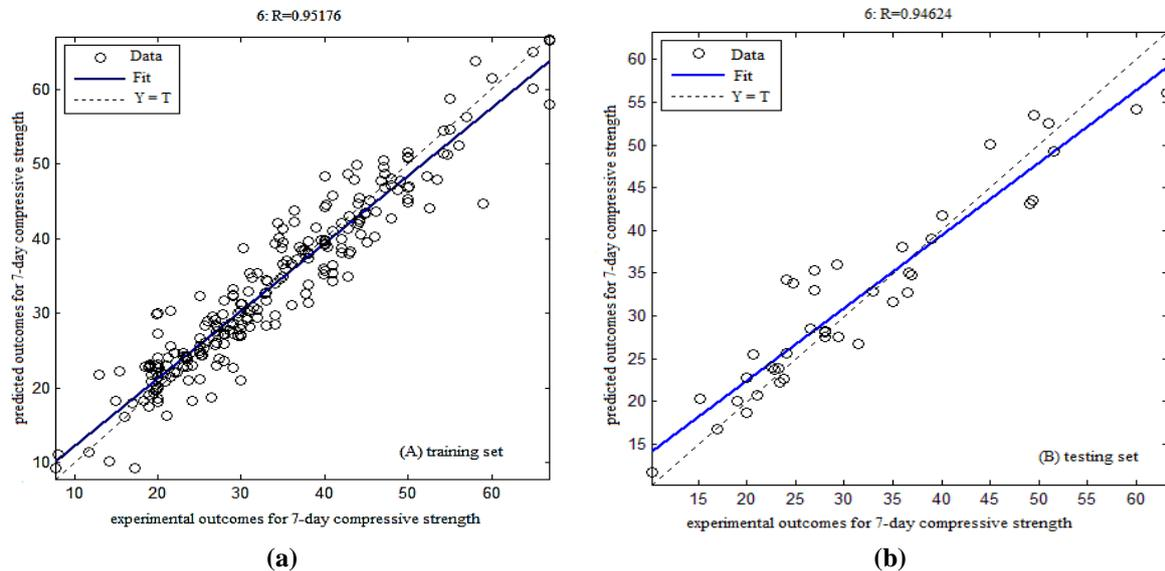
**Fig. 4.** Predicted outcomes vs. experimental outcomes for 7-day compressive strength: a) Training set and; b) Testing set
