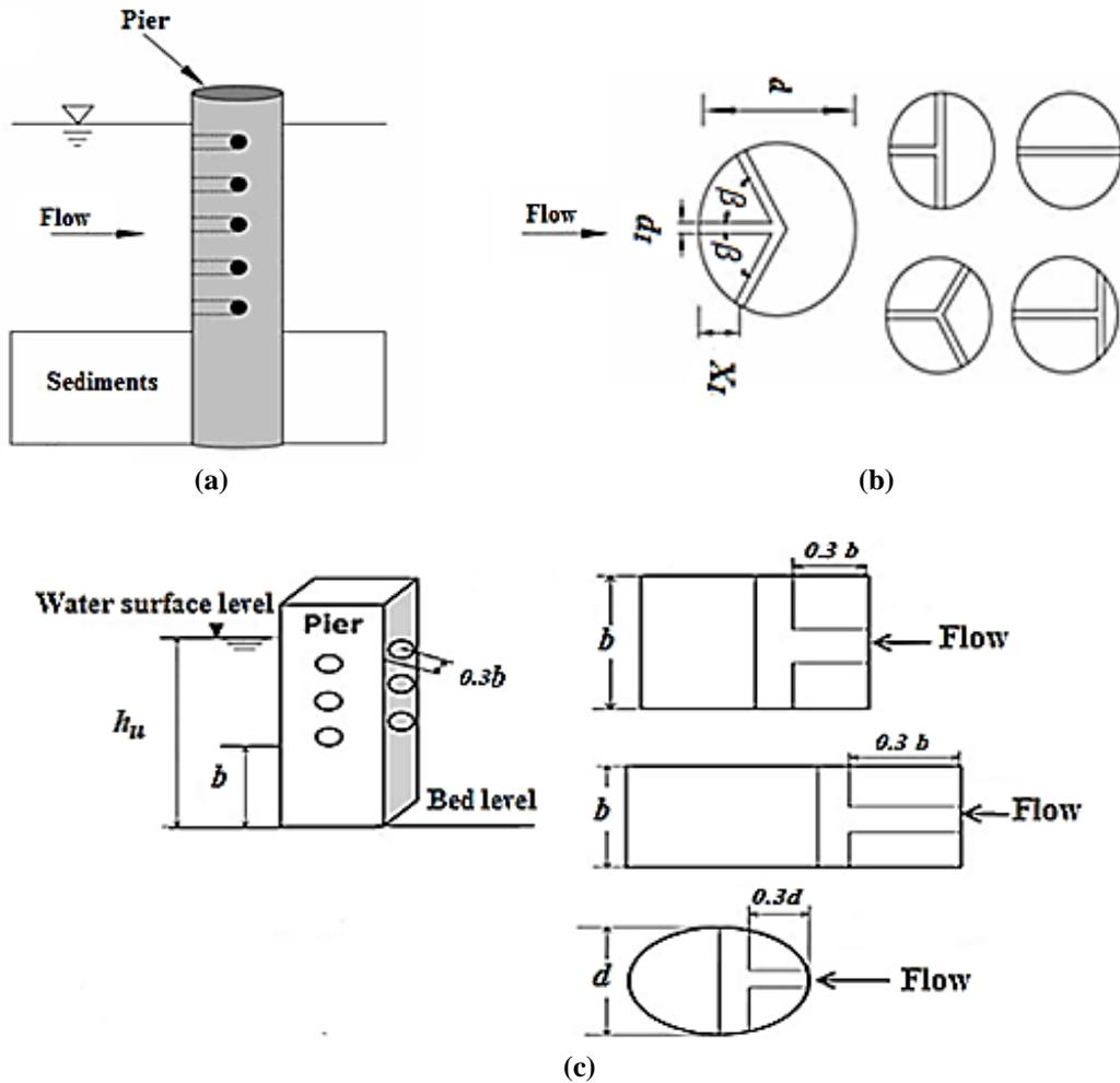
**Fig. 2.** Schematic diagram of internal connecting tubes: a) Side view; b) Typical cross-sections (Redrawn from Abd El-Razek et al., 2003) and; c) Different pier shapes and opening arrangement (Redrawn from Entesar et al., 2013)
