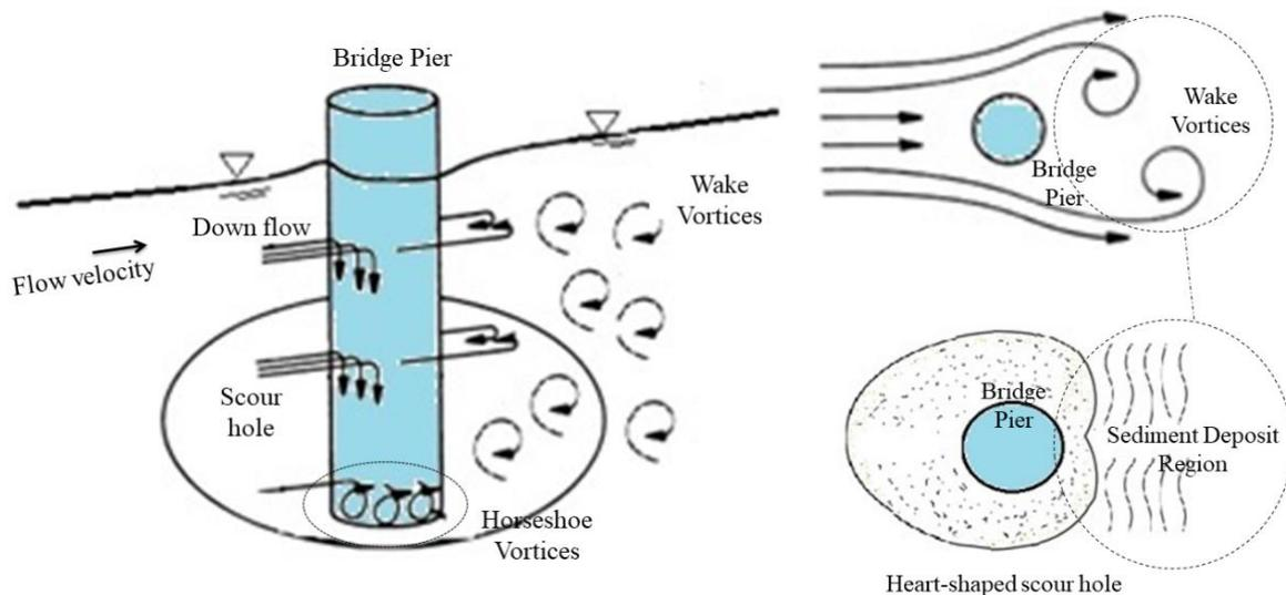
**Fig. 1.** Schematic diagram of developed scour hole, horseshoe and wake vortices, and heart shaped scour hole
