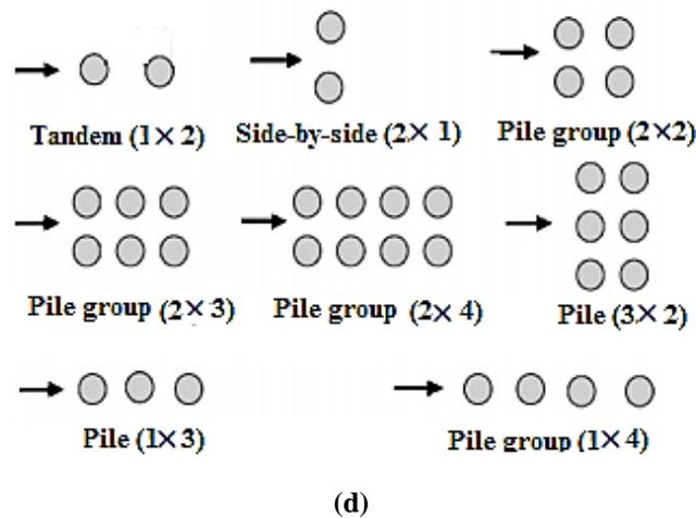
**Fig. 3.** a) Schematic representation of partial pier group including side view, and cross sections (Redrawn from Vittal et al., 1994 and Ezzeldin et al., 2006); b) The different of array configurations of seven smaller piers (Redrawn from Yagci et al., 2017); c) Five orientations of the twin-pile group (Redrawn from Liang et al., 2012) and; d) Pile groups used in experiments (Redrawn from Ataie-Ashtiani and Beheshti, 2006)
