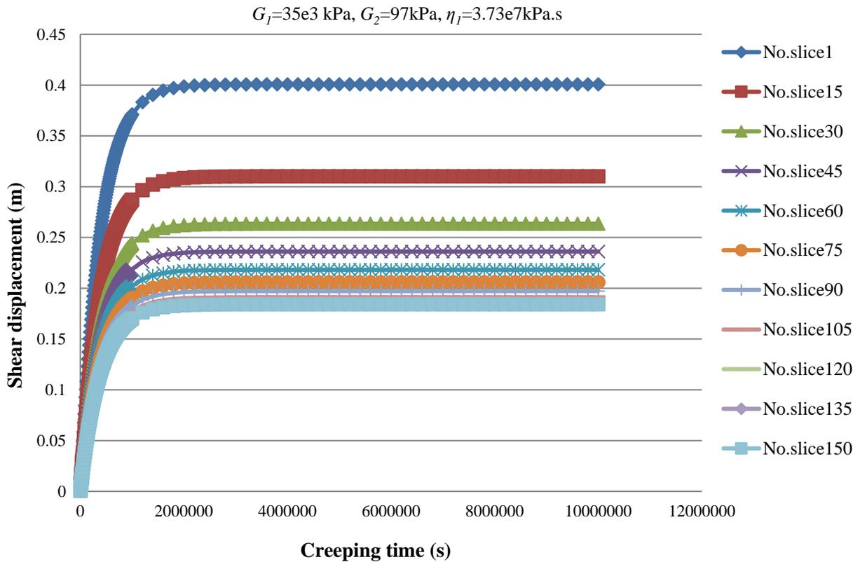
Fig. 9. Shear displacement of visco-elastoplastic points on the surface sliding with creeping time using the proposed method for different slices
