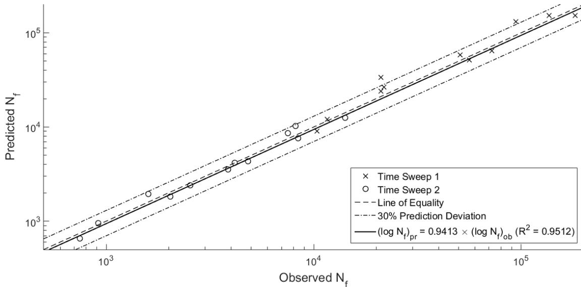
**Fig. 6.**  $N_f$  acquired from validation tests (observed) and the developed method (predicted)
