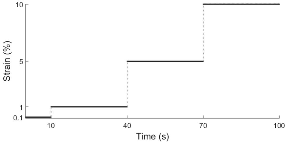
Fig. 3. Strain pattern of loadings at frequency of 10 (Hz)
