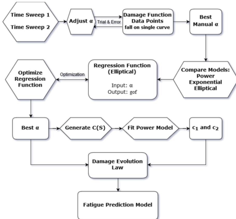
Fig. 4. Flowchart diagram of the new procedure to obtain fatigue prediction model
