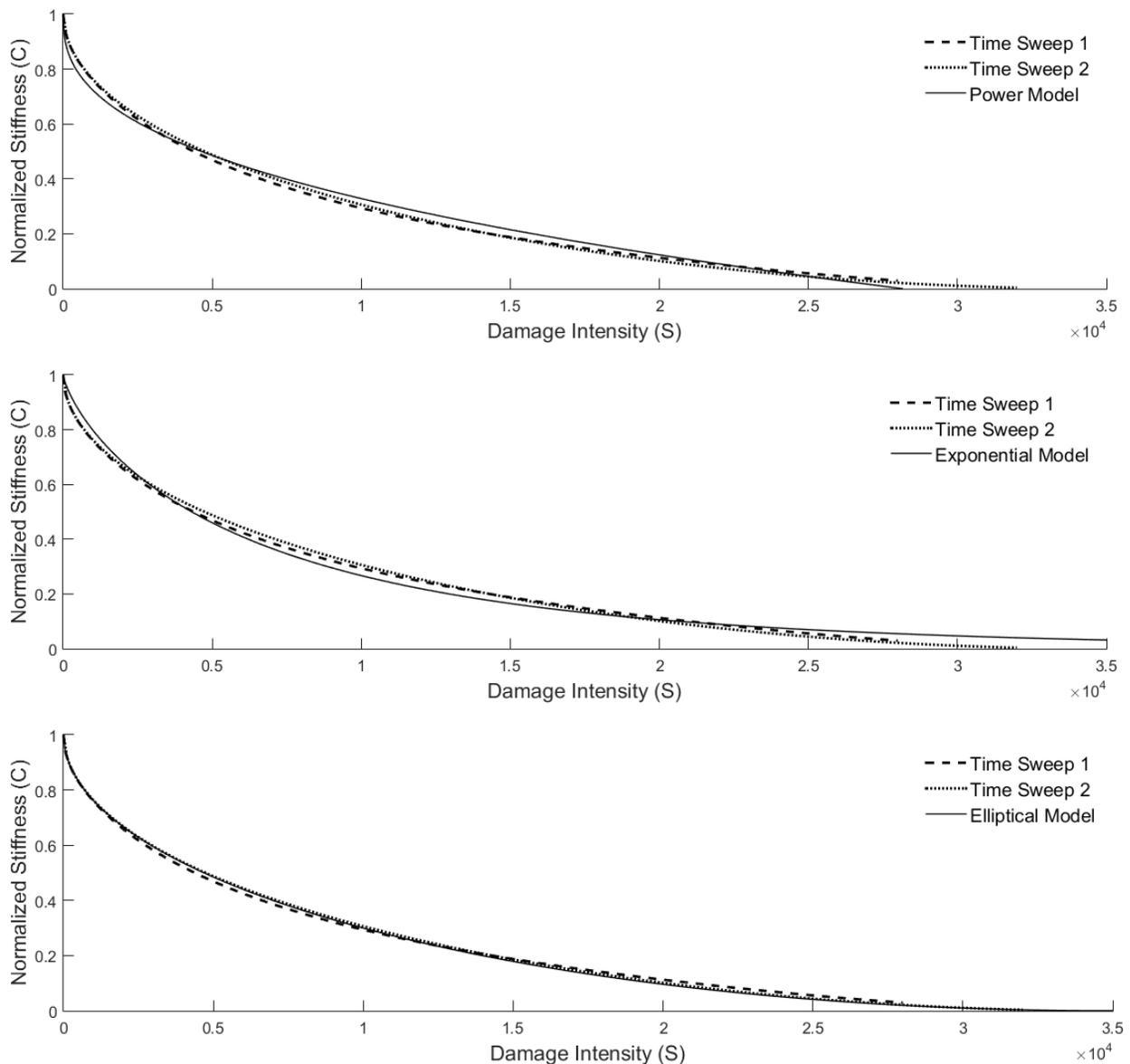
**Fig. 2.** General shape of the three models, and the conformity with data points of damage function (binder sample S24 at 15 °C)
