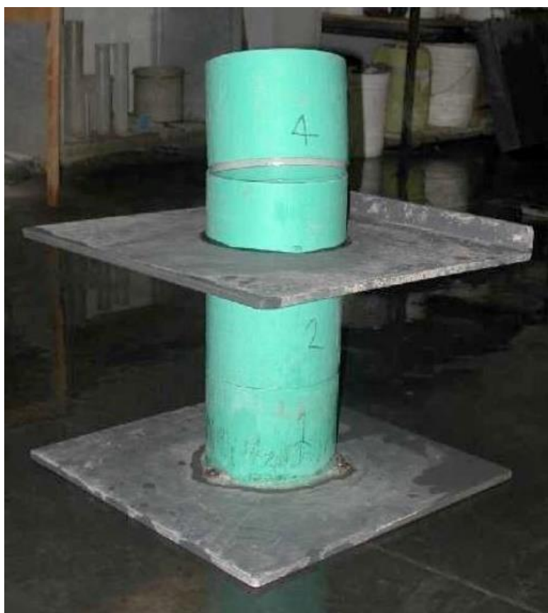
Fig. 1. Photo of the column segregation test
