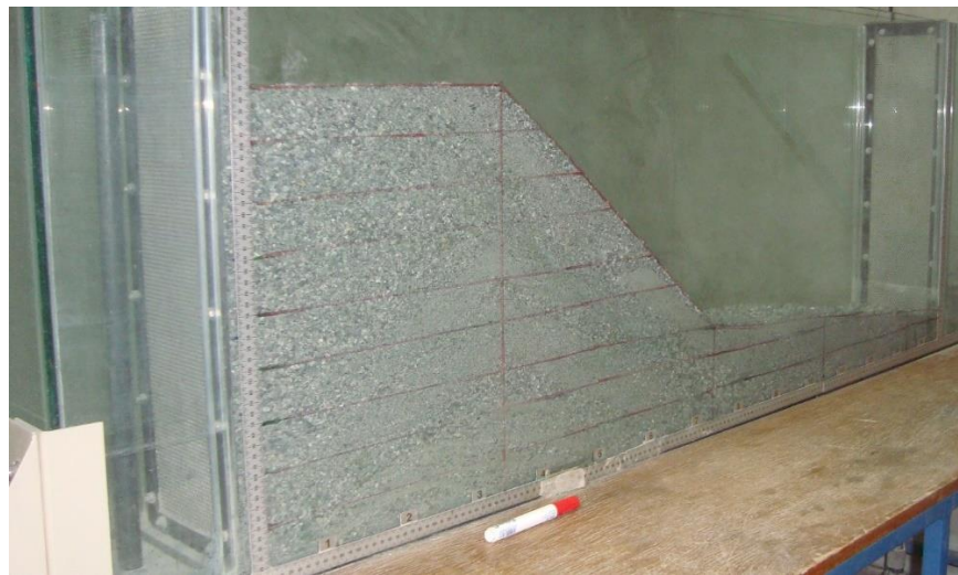
Fig. 5. Unreinforced slope modeled in test box
