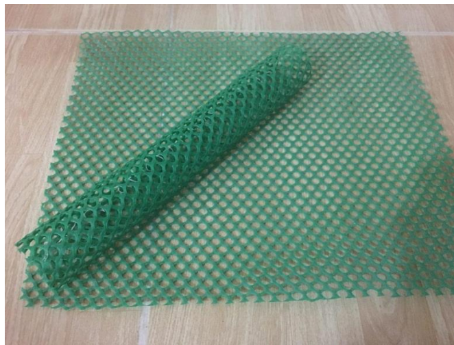
Fig. 3. Geogrid layer used in experimental modeling
