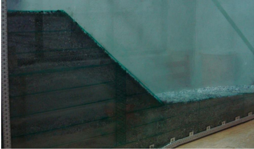
Fig. 8. OSC reinforced slope modeled in test box
