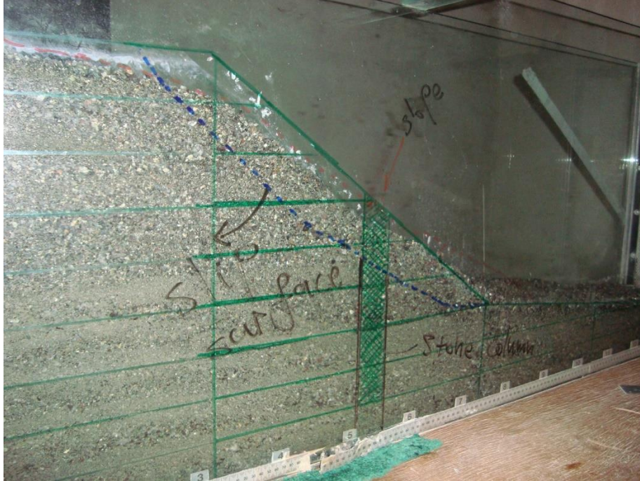
Fig. 10. Failure of OSC reinforced slope under overburden stress of 6.26 kPa
