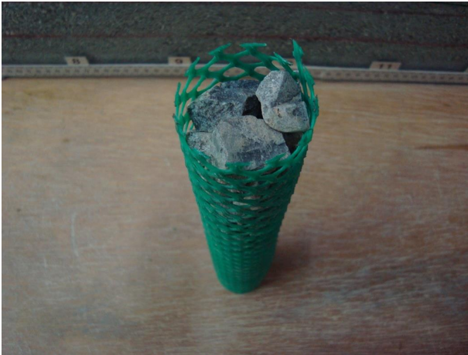
Fig. 11. Geogrid Encased Stone Column (GESC)
