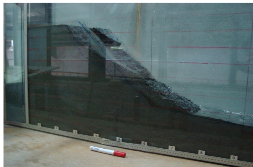
Fig. 6. Failure of unreinforced slope due to saturation
