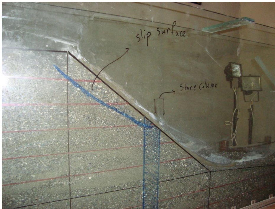
Fig. 13. Failure of GESC reinforced slope under overburden stress of 13.59 kPa
