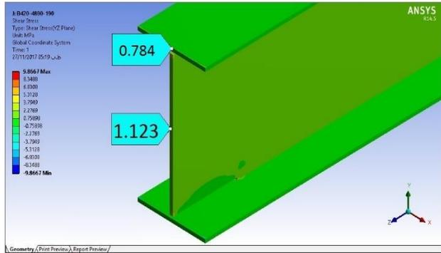
Fig. 19. Shear stress in model B420-4800-190
