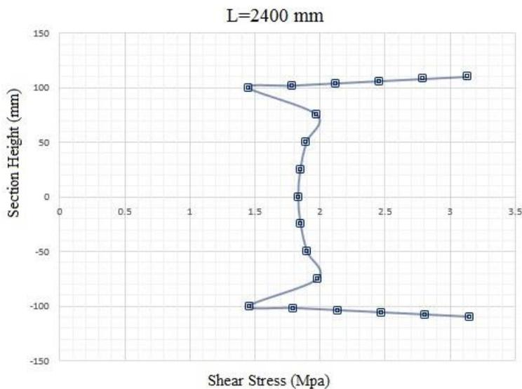
Fig. 9. Shear stress distribution at the cross section height in model B220-2400-0
