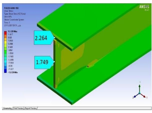
Fig. 17. Shear stress in model B220-6000-190
