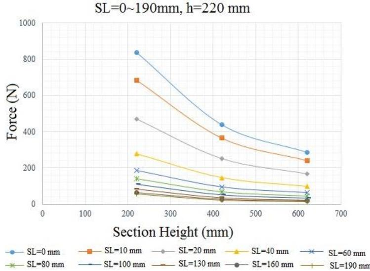
Fig. 24. Change of flange shear force from section total shear with change of beam section height for models Ba-3600-0 to Ba-3600-190 (a = 220, 420 and 620 mm)
