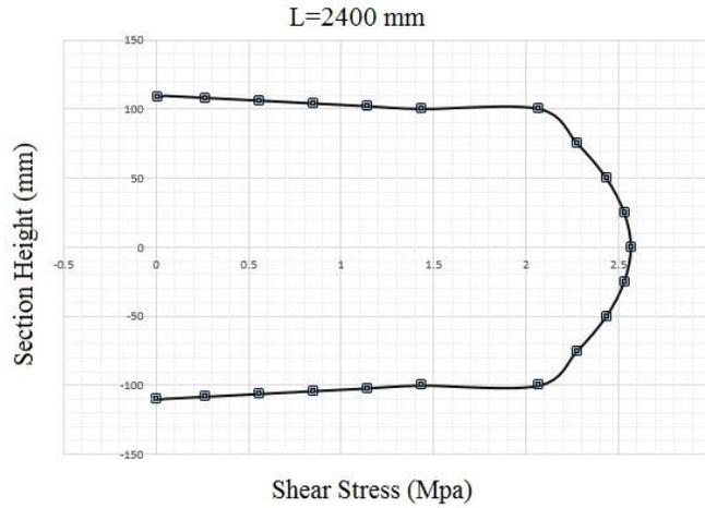
Fig. 10. Vertical shear stress distribution in model B220-2400-0 at a distance of 200 mm from support
