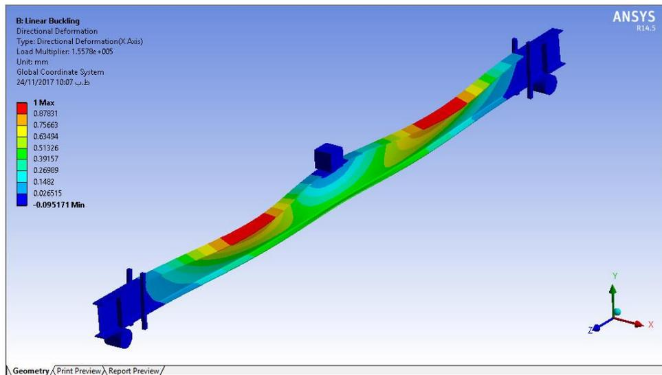
Fig. 6. Sine wave deformation of model P210 in validation
