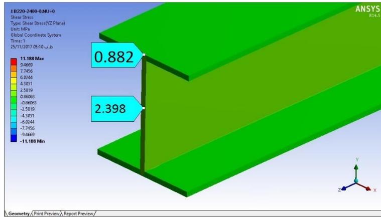
**Fig. 28.** Shear stress in model B220-2400-0,  $\vartheta = 0$
