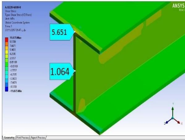
Fig. 16. Shear stress in model B220-6000-0
