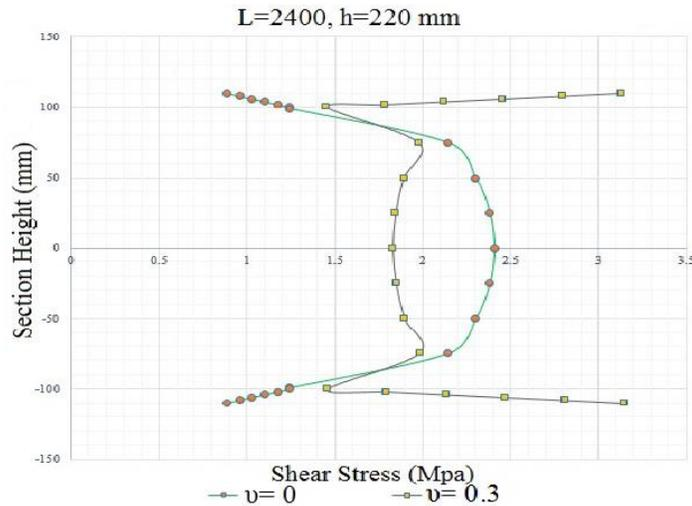
**Fig. 26.** Vertical shear distribution at connection section in the beam with transverse strains ( $\nu=0.3$ ) and without transverse strains ( $\nu = 0$ ) in model B220-2400-0
