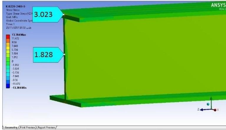
**Fig. 27.** Shear stress in model B220-2400-0,  $\vartheta = 0.3$
