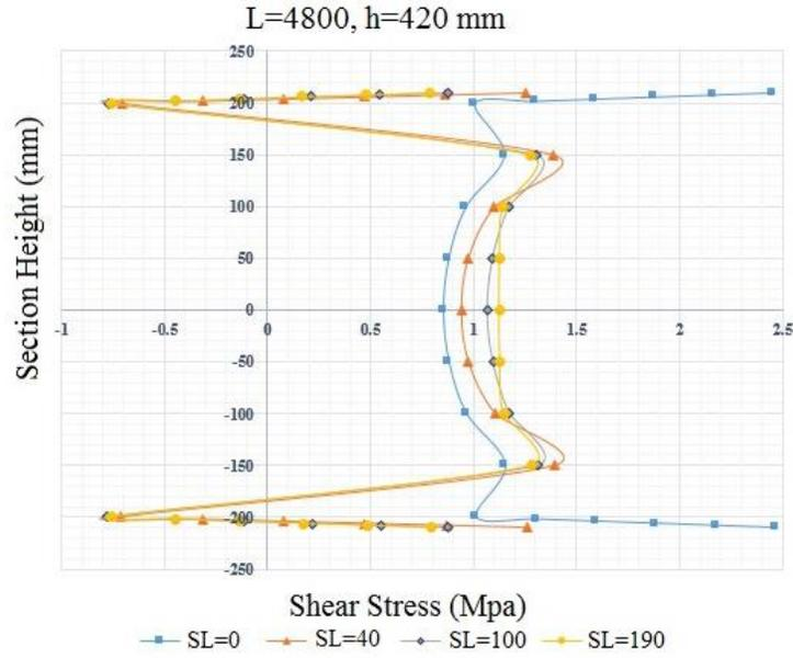
Fig. 13. The effect of increasing slot length on vertical shear stress distribution at section height
