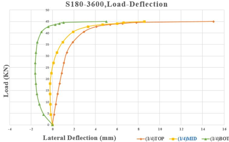
Fig. 8. Load–deflection curve of model P180 for validation
