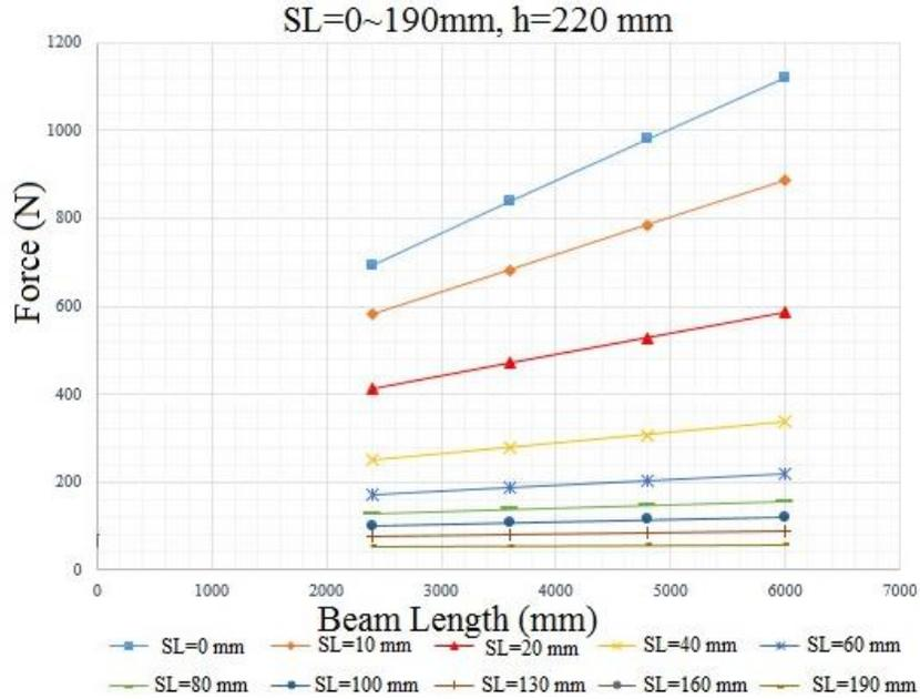
Fig. 22. Change of flange shear force from section total shear with change of beam span length for models B220-b-0 to B220-b-190 (b = 2400, 3600, 4800 and 6000 mm)
