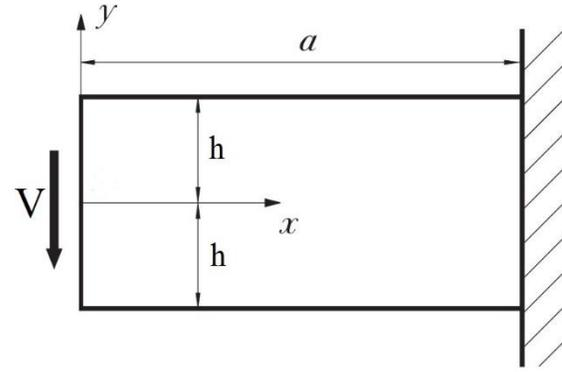
Fig. 1. Cantilever with an end load
