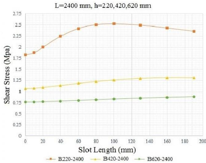
Fig. 11. The effect of slot length on increasing neutral axis shear stress
