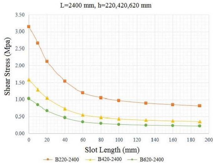
Fig. 12. The effect of slot length on decreasing outer fiber shear stress
