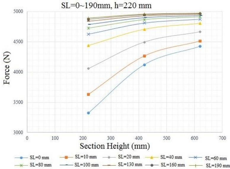
Fig. 25. Change of flange shear force from section total shear with change of beam section height for models Ba-3600-0 to Ba-3600-190 (a = 220, 420 and 620 mm)
