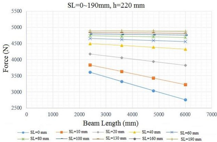
Fig. 23. Change of web shear force from section total shear with change of beam span length for models B220-b-0 to B220-b-190 (b = 2400, 3600, 4800 and 6000 mm)
