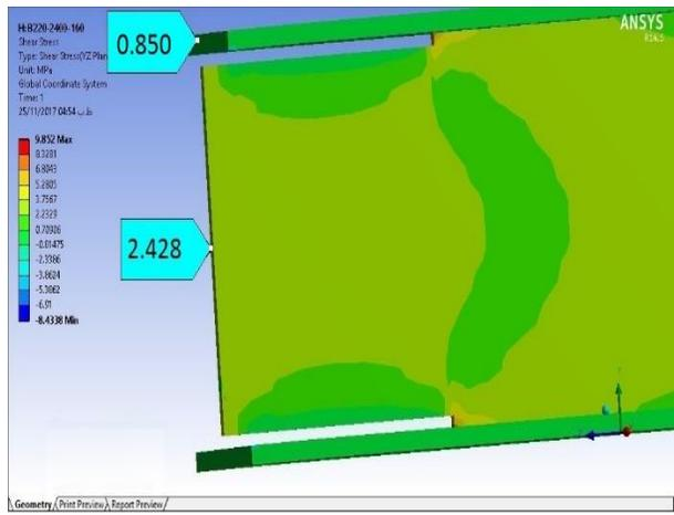
Fig. 15. Shear stress in model B220-2400-160
