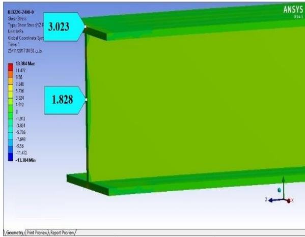
Fig. 14. Shear stress in model B220-2400-0
