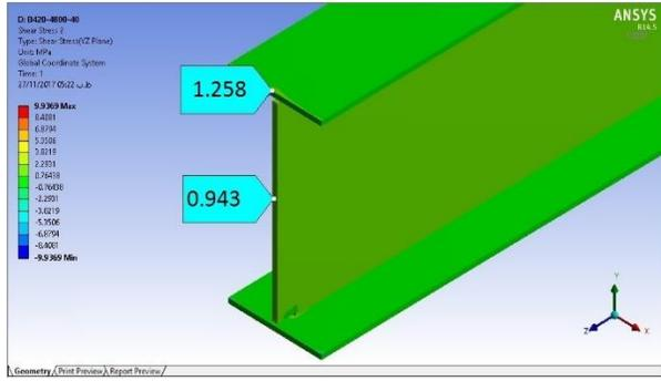
Fig. 18. Shear stress in model B420-4800-40
