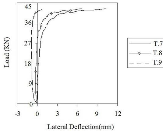
Fig. 7. Load-deflection curve of model P180 in Zirakian's experimental research
