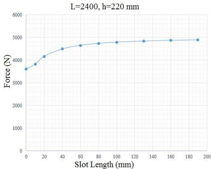
**Fig. 21.** The portion of web from total shear force at connection section by increasing slot length in models B220-2400-0 to B220-2400-190
