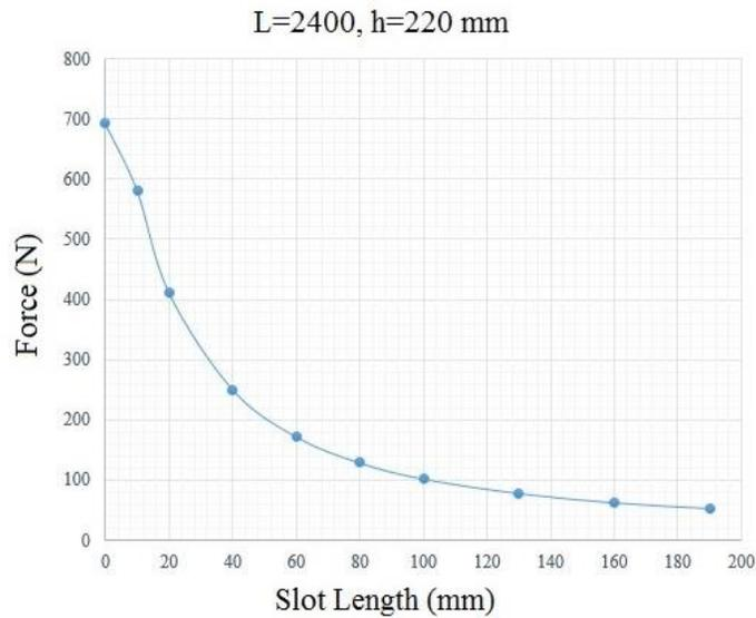
**Fig. 20.** The portion of top (bottom) flange from total shear force at connection section by increasing slot length in models B220-2400-0 to B220-2400-190
