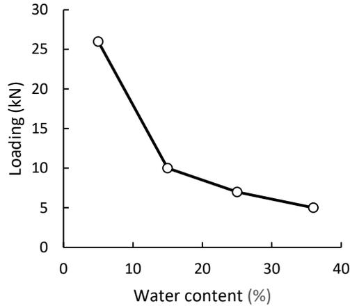
Fig. 12. The effect of percentage of lime mortar moisture on strength of CLM column specimens
