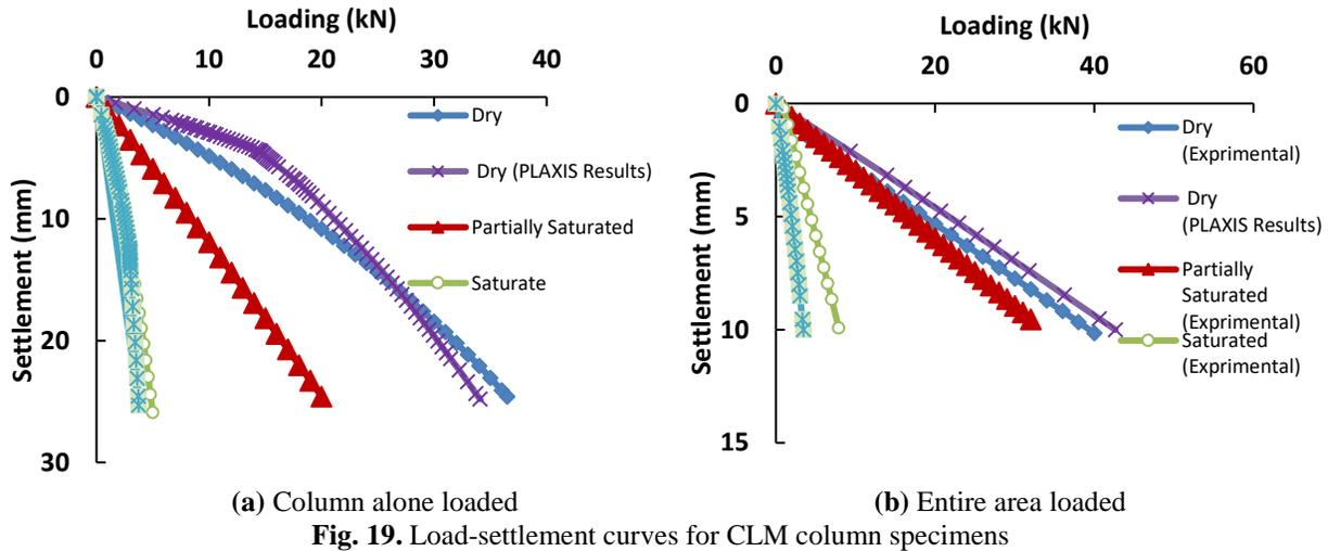
Fig. 19. Load-settlement curves for CLM column specimens
