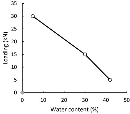
**Fig. 10.** The effect of percentage of moisture on clayey specimen's strength
