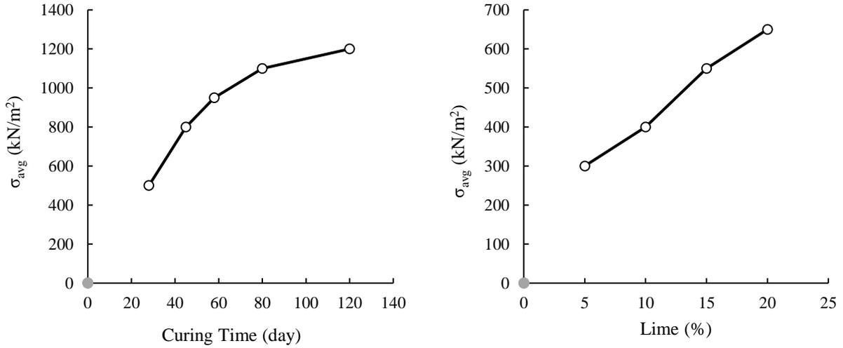
a) Relationship between compressive strength of lime mortar and curing time      b) Relationship between compressive strength of lime mortar and lime content
