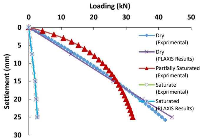
**Fig. 18.** Load-settlement curves for clay specimens
