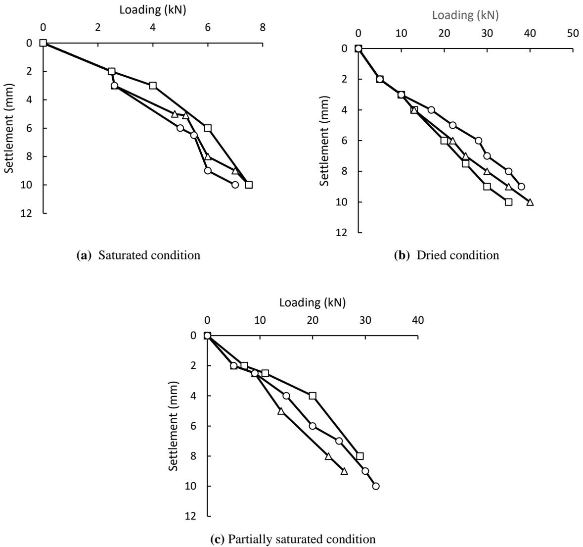
Fig. 13. Load-settlement behavior of CLM column specimen (entire area loaded)
