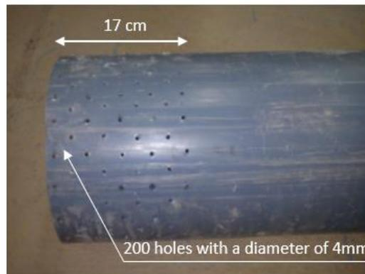
Fig. 2. Perforated polyethylene pipe
