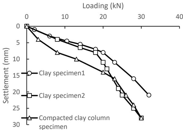
Fig. 16. Load-settlement behavior of compacted clay column (column alone loaded) specimen and clay specimens
