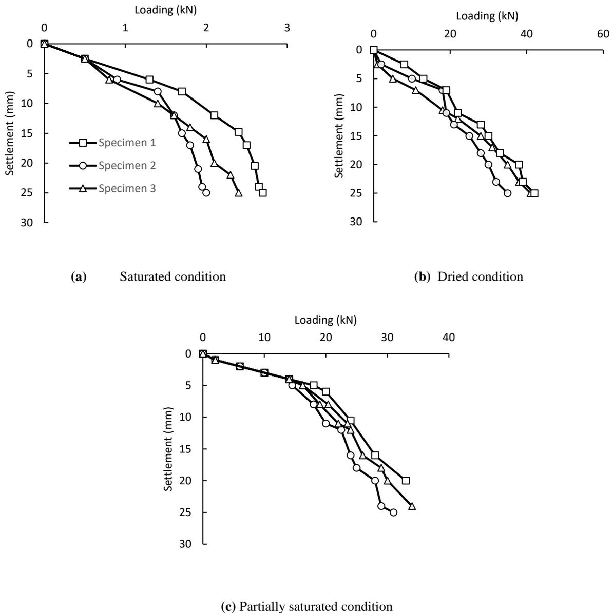
**Fig. 9.** Load-settlement behavior of untreated layered soils
