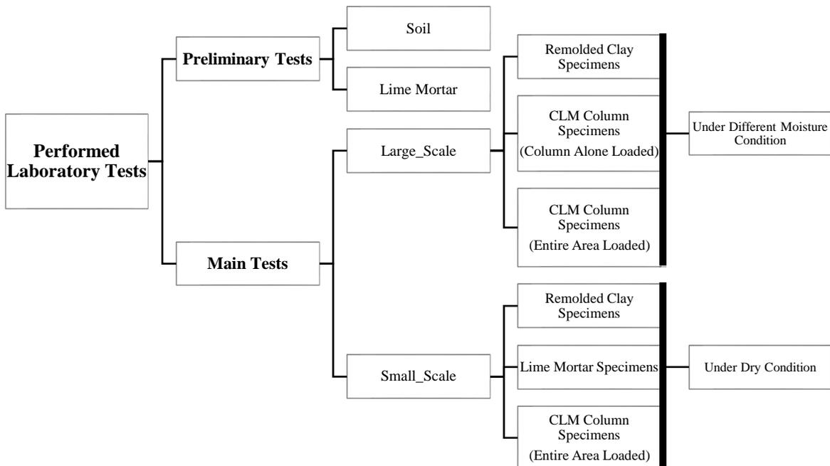
Fig. 1. Overview of performed laboratory tests
