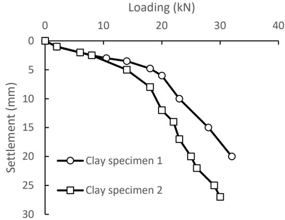
Fig. 14. Load-settlement behavior of clay specimens
