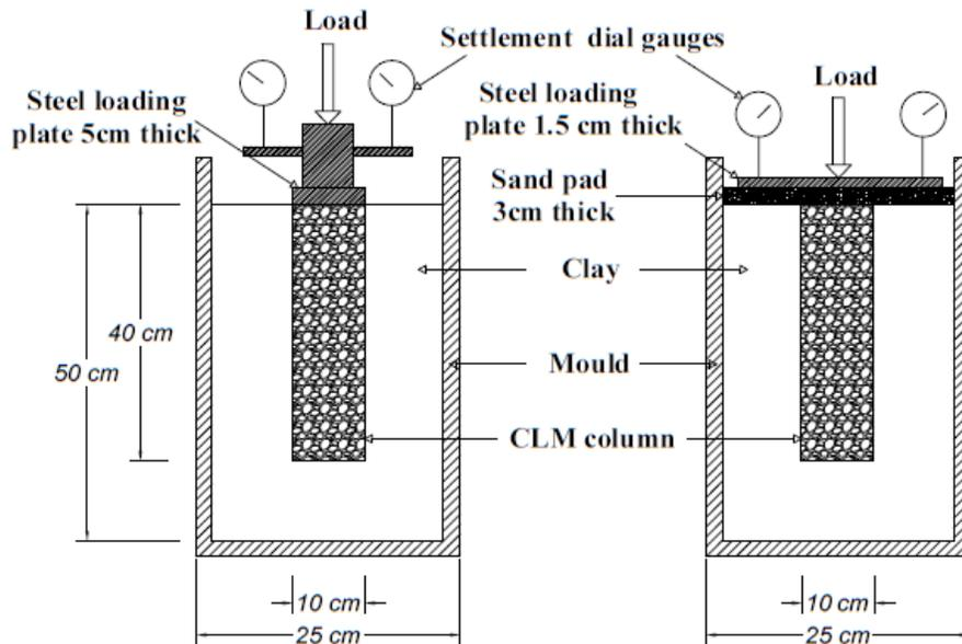
(a) CLM column Specimen (Column alone loaded) (b) CLM column specimen (Entire area loaded)
