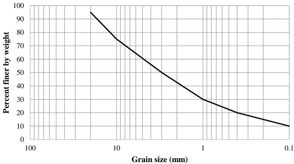
**Fig. 4.** Grain size distribution of well-graded sand
