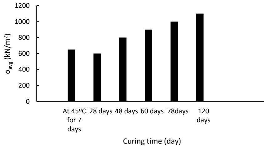
**Fig. 8.** Influence of temperature on curing time
