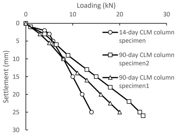
Fig. 15. Load-settlement behavior of CLM column (column alone loaded) specimens
