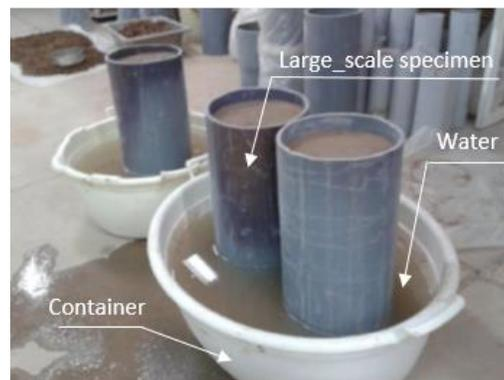
Fig. 3. Capillary process for saturating the specimens
