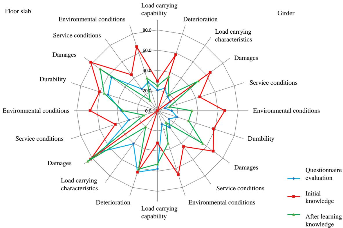
Fig. 11. Visualized comparison of bridge girder and floor slab performance evaluation results (in case of Span 1)
