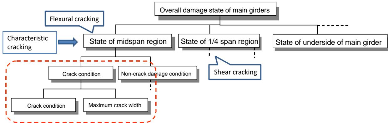
Fig. 4. Example of performance evaluation based on hierarchical criteria in RC-BREX system
