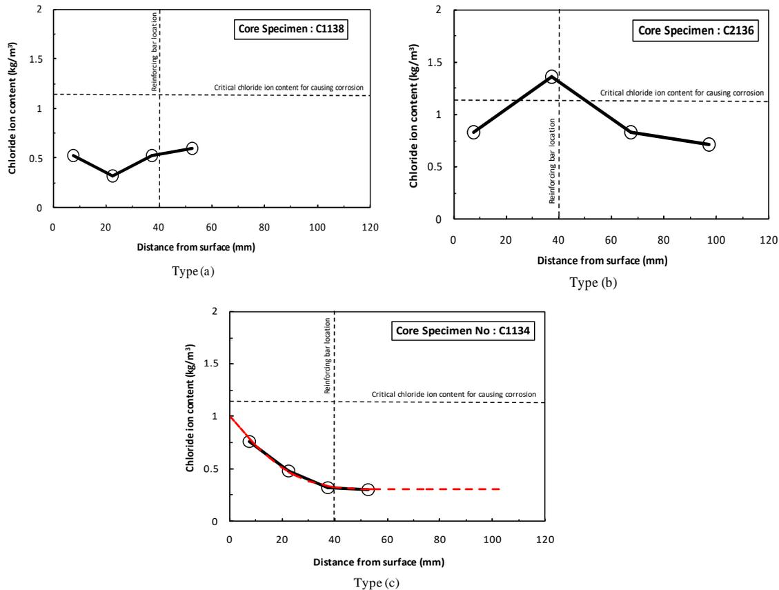
**Fig. 14.** Types of chloride ion content distribution
