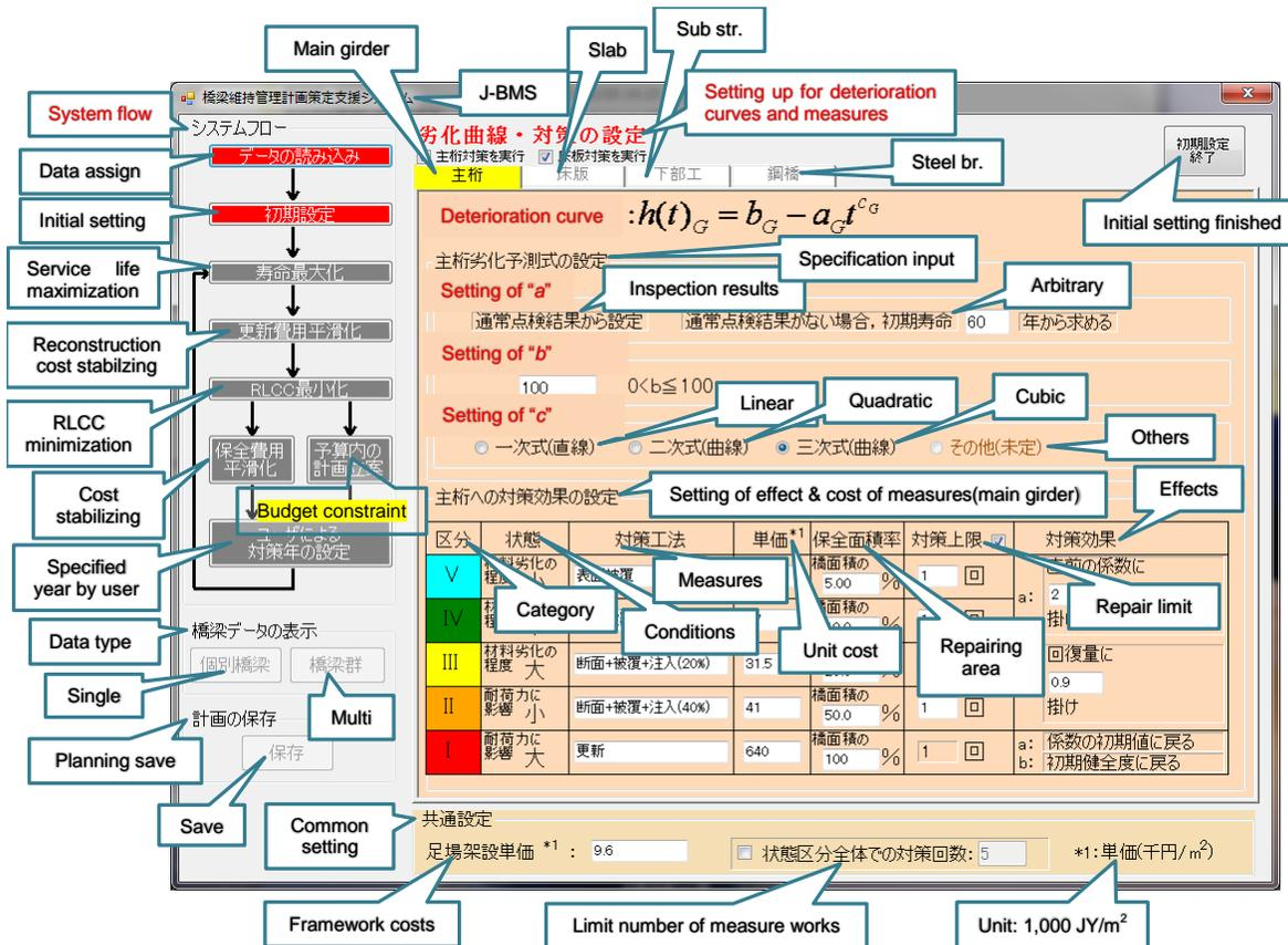
Fig. 5. Example of initial setting screen for deterioration curve predicting parameters (in Japanese system)
