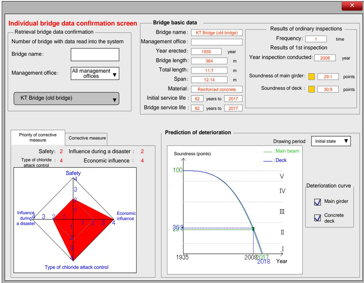
Fig. 6. Example of service life maximization function of MPOS (after reconstruction cost spreading)
