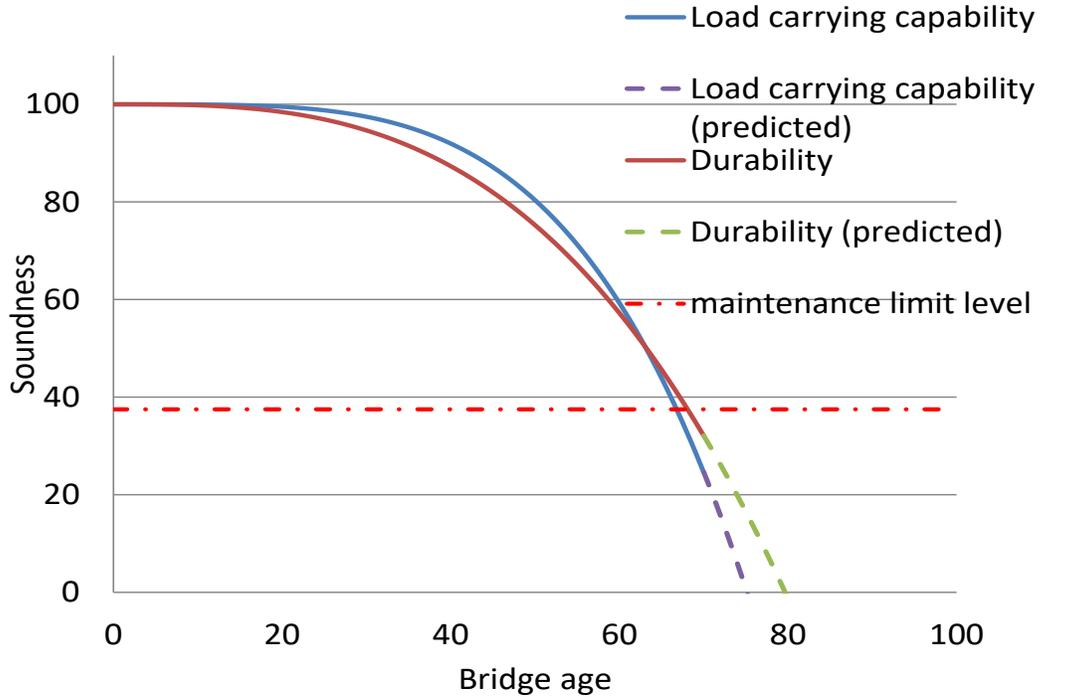
(a) Deterioration prediction curve for main girder
