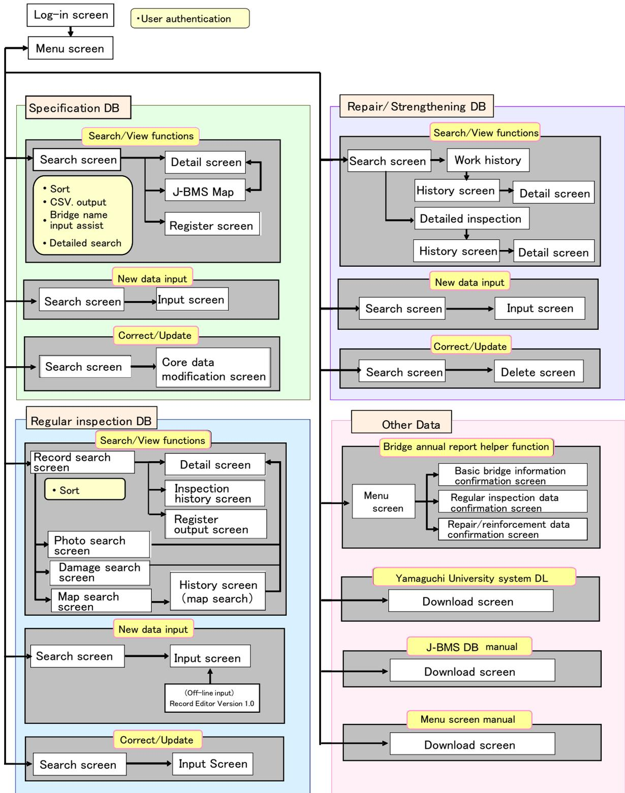
Fig. 3. Whole configuration of J-BMS DB '09
