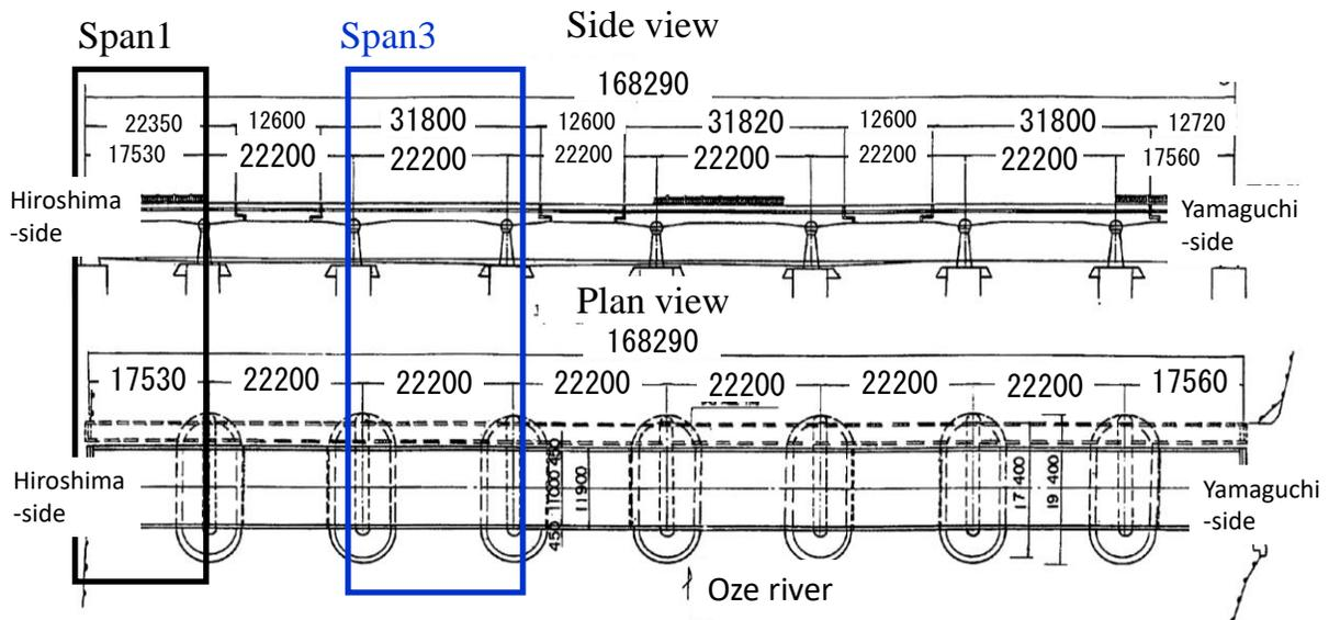
**Fig. 7.** Side and plan views of SK-Bridge (before removal) and inspection area (span) (unit: mm)
