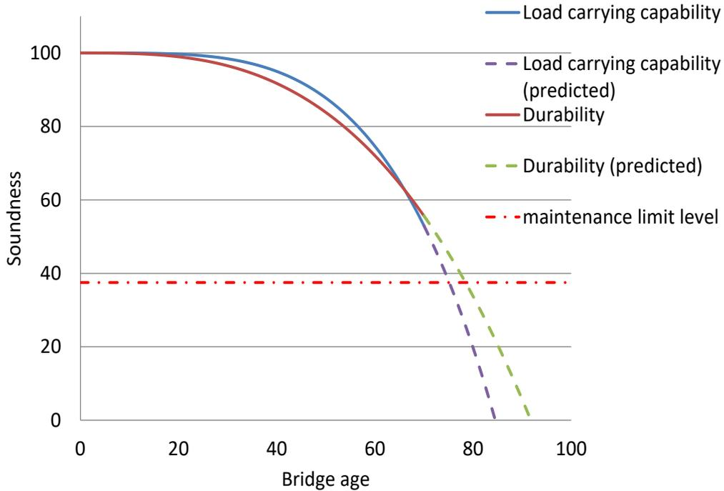
(b) Deterioration prediction curve for floor slab
