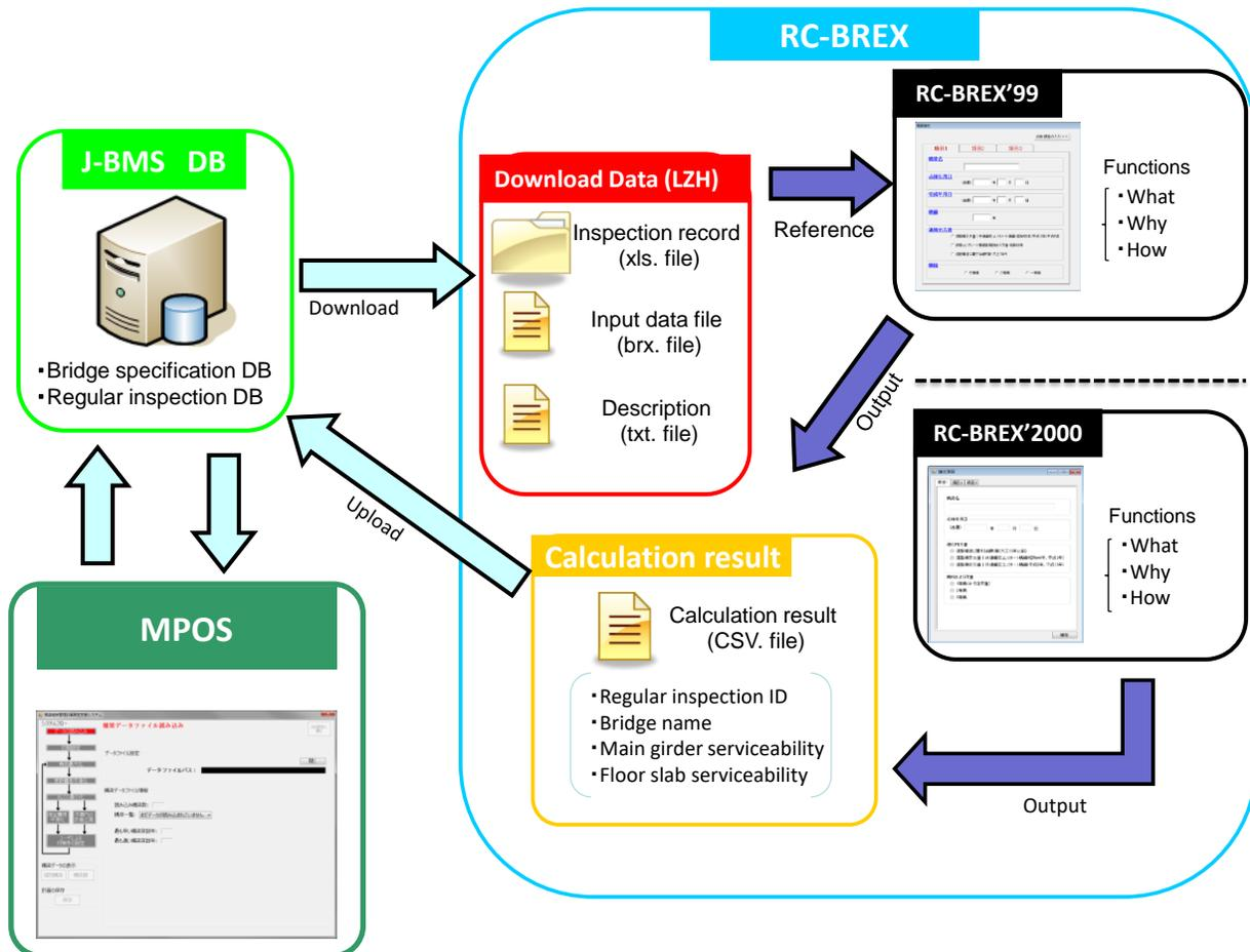
Fig. 2. Operation flow of J-BMS RC version
