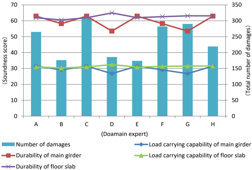
Fig. 10. Total number of damages and performance evaluation results for SK-Bridge by domain experts
