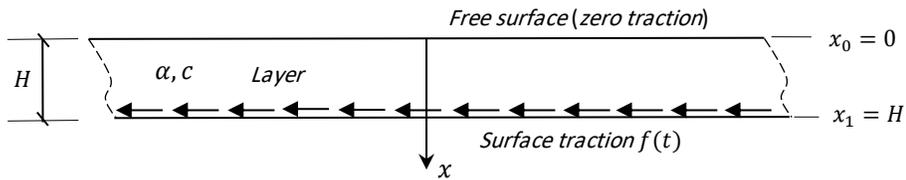
Fig. 3. A single layer subjected to an arbitrary traction at the bottom
