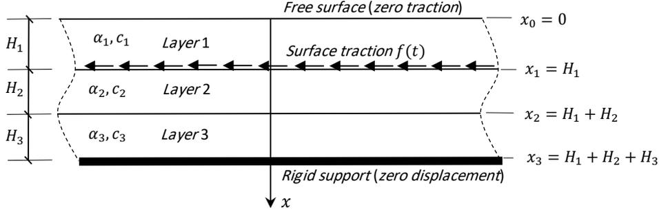
Fig. 2. A three-layered elastic medium subjected to an arbitrary time-dependent traction
