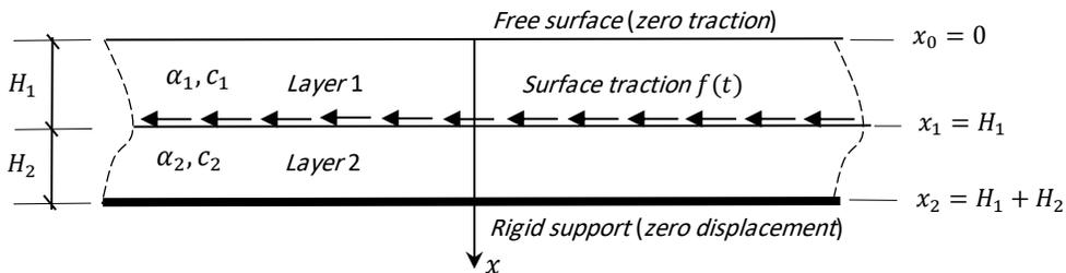
Fig. 5. A two-layered medium fixed at the bottom and subjected to an arbitrary traction at the interface
