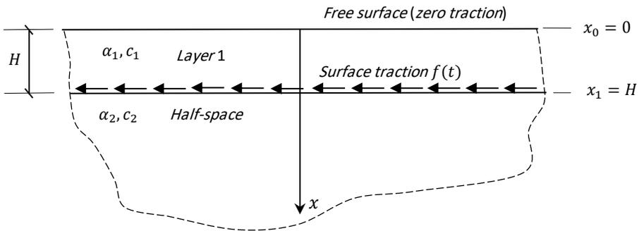
Fig. 4. A single layer rested on the top of a half-space subjected to an arbitrary traction at the interface
