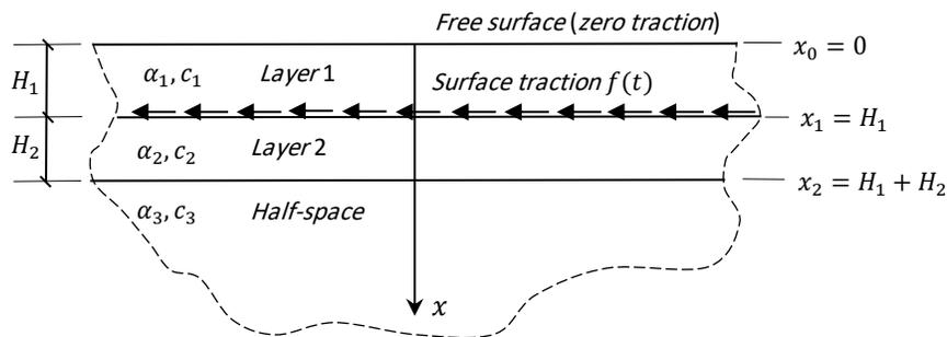
**Fig. 6.** Two elastic layers resting on an elastic half-space subjected to an arbitrary traction at the bottom of the first layer
