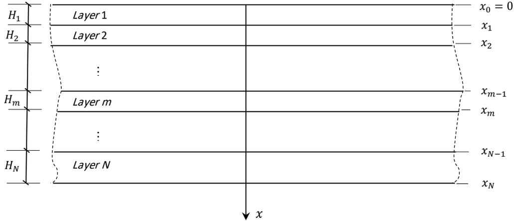
Fig. 1. A multi-layered one-dimensional elastic medium
