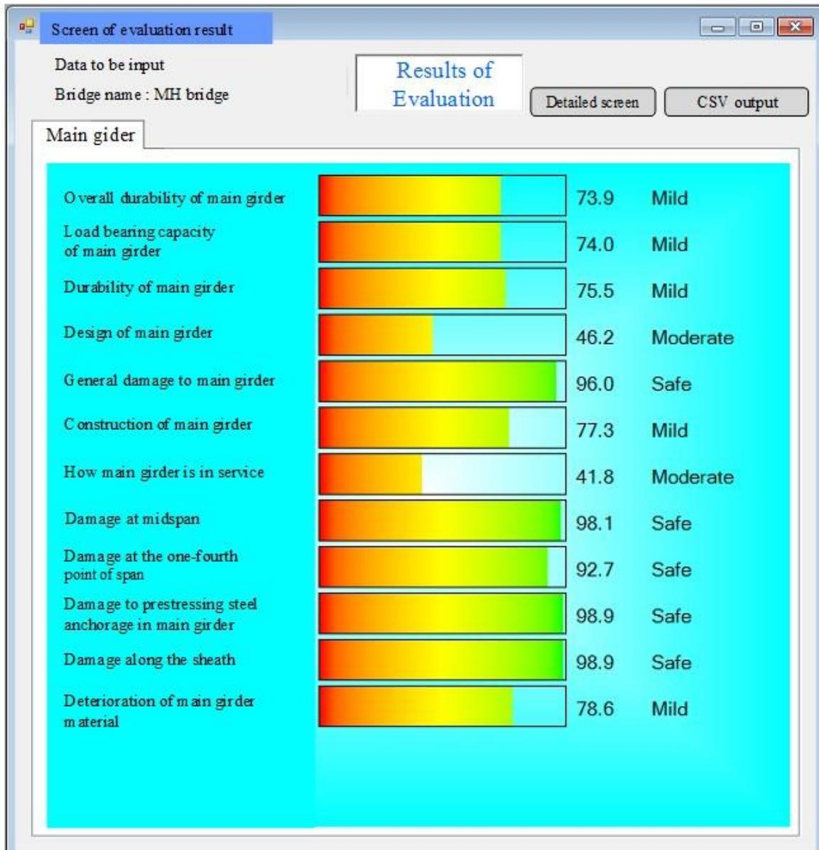
Fig. 3. Sample screen showing evaluation results for parameters of main girder
