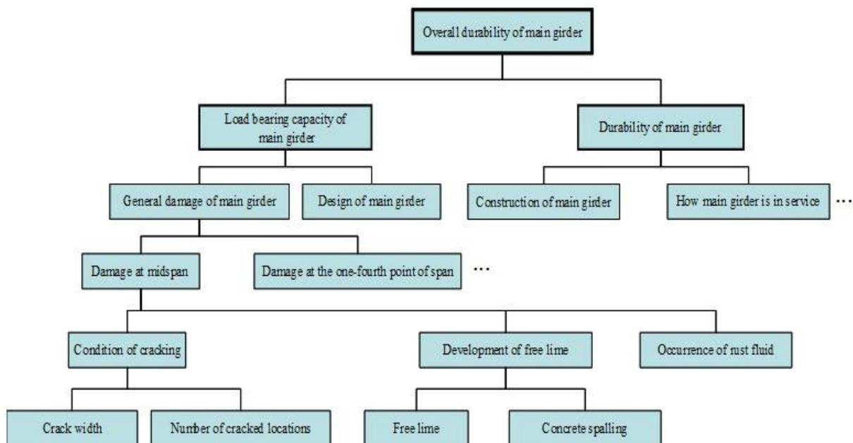
**Fig. 2.** Part of the process of evaluating overall durability of main girder
