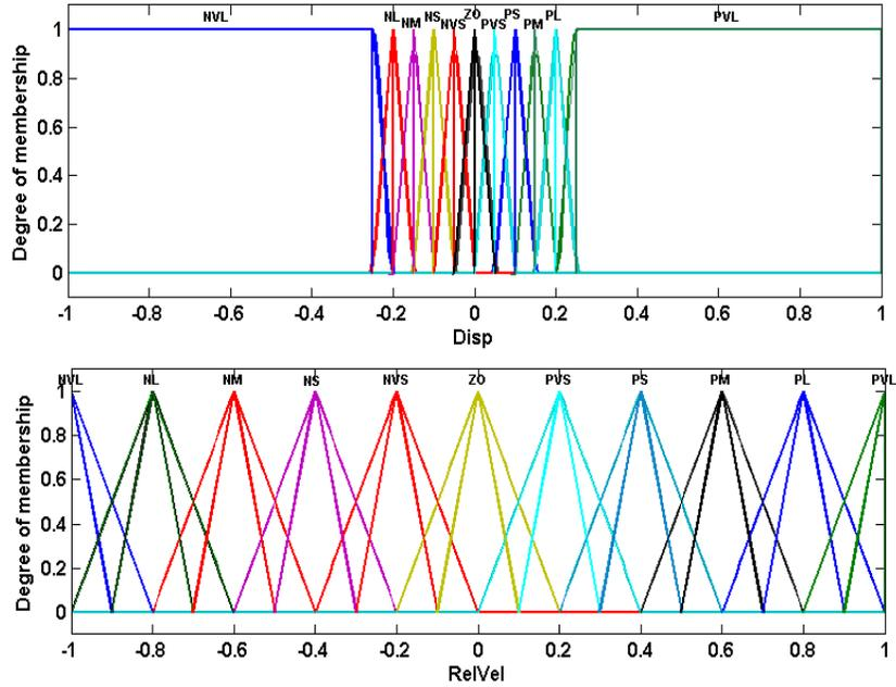
Fig. 10. Input and output membership functions for type-2 FLC
