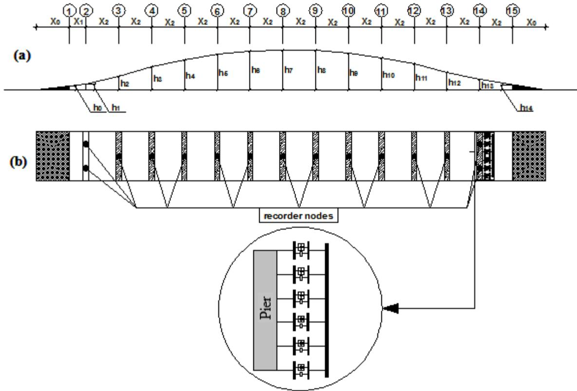
Fig. 1. a) Side view, b) Top view of the College bridge and details of the MR dampers' placement
