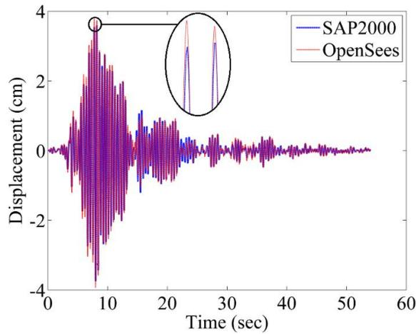
Fig. 3. Longitudinal displacement of the tallest pier (pier 9) subjected to Kern-County earthquake
