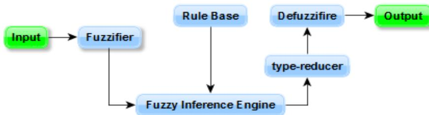
Fig. 8. The schematic diagram of the type-2 FLC
