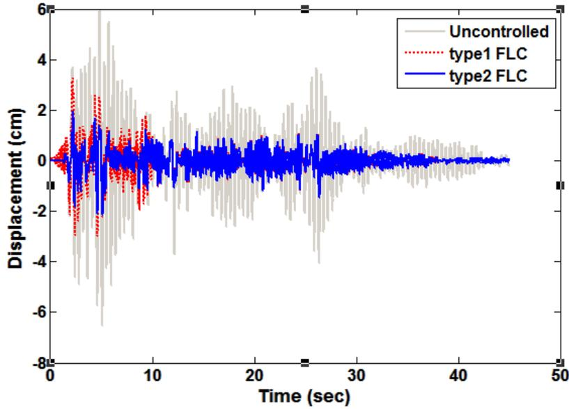
Fig. 12. Displacement time history of the largest pier of bridge
