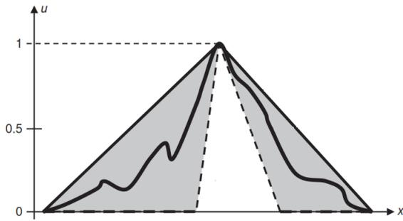
Fig. 22. The membership functions of the type-2 FLCs
