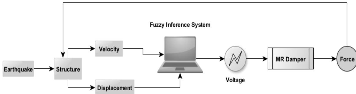
**Fig. 11.** Process of the devised semi-active control system
