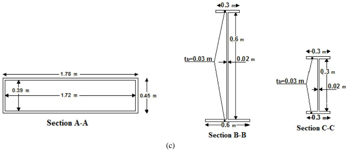
Fig. 2. a) Front view, b) Side view, c) Cross sections of a typical pier of the bridge
