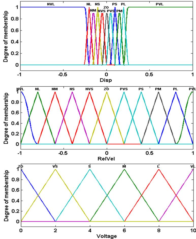
Fig. 9. Input and output membership functions for type-1 FLC
