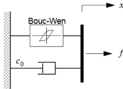
Fig. 4. Mechanical Model of the MR Damper
