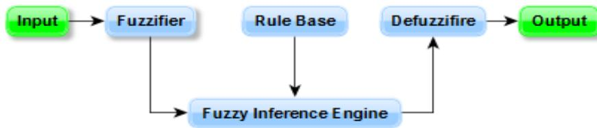
Fig. 7. The schematic diagram of the type-1 FLC
