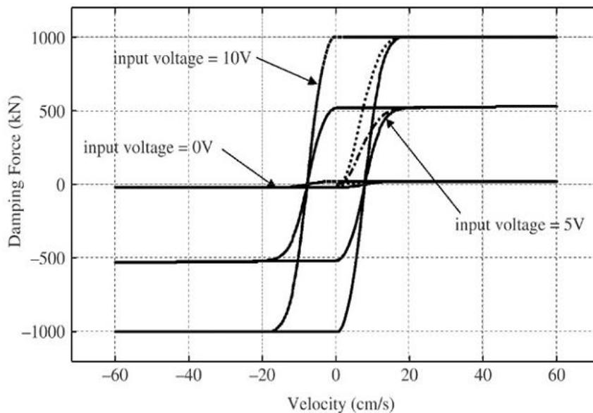
Fig. 5. Mechanical behavior of MR damper, presented by Ok et al. (2007)
