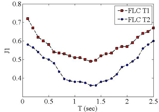
Fig. 23. Variations of  $J_1$  versus natural period of an SDOF structure for type-1 and type-2 FLC
