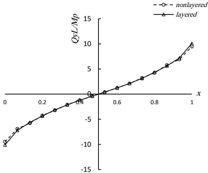
**Fig. 16.** Shear force diagram at the middle cross section ( $y = 0.5$ ) corresponding to  $PL^2/M_p = 24$  (clamped plate subjected to uniformly distributed load)
