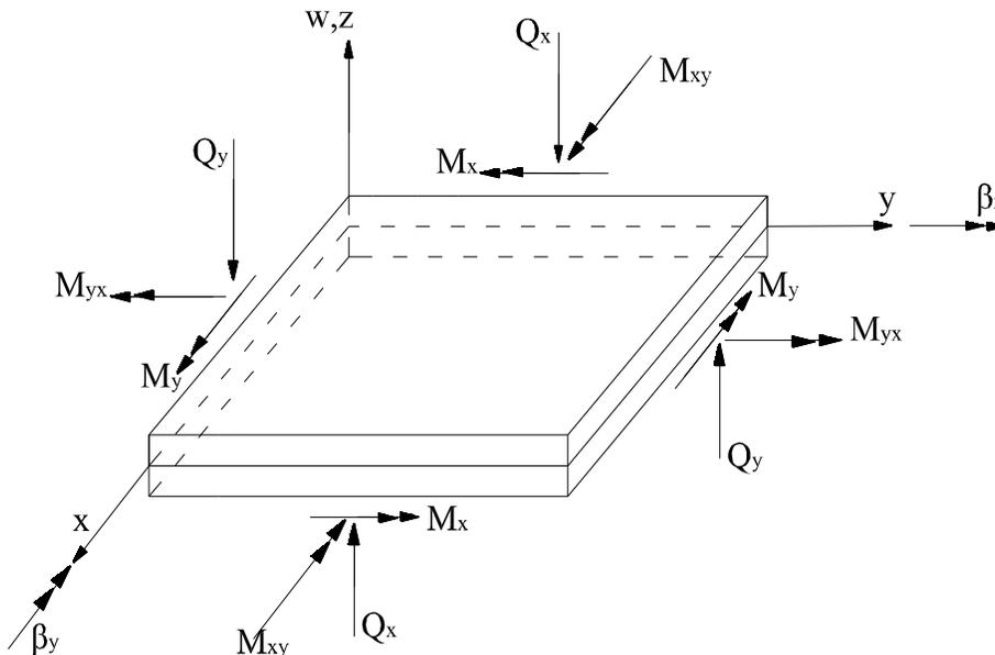
Fig. 1. Sign convention of the moment, shear force, and section rotation
