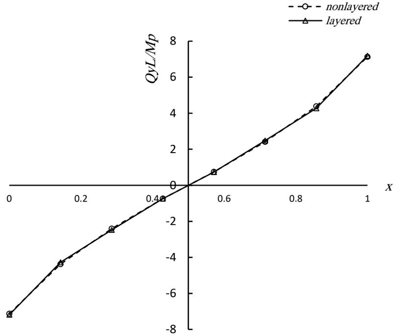
**Fig. 9.** Shear force diagram at the middle cross section ( $y = 0.5$ ) corresponding to  $PL^2/M_p = 20.7$  (simply supported plate subjected to a uniformly distributed load)
