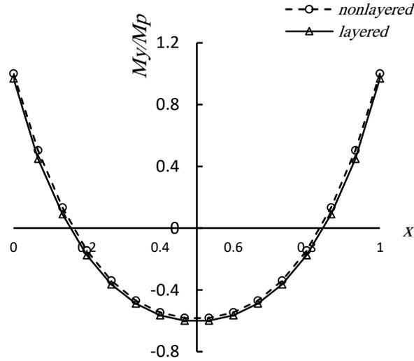
**Fig. 15.** Moment diagram at the middle cross section ( $y = 0.5$ ) corresponding to  $PL^2/M_p = 24$  (clamped plate subjected to uniformly distributed load)
