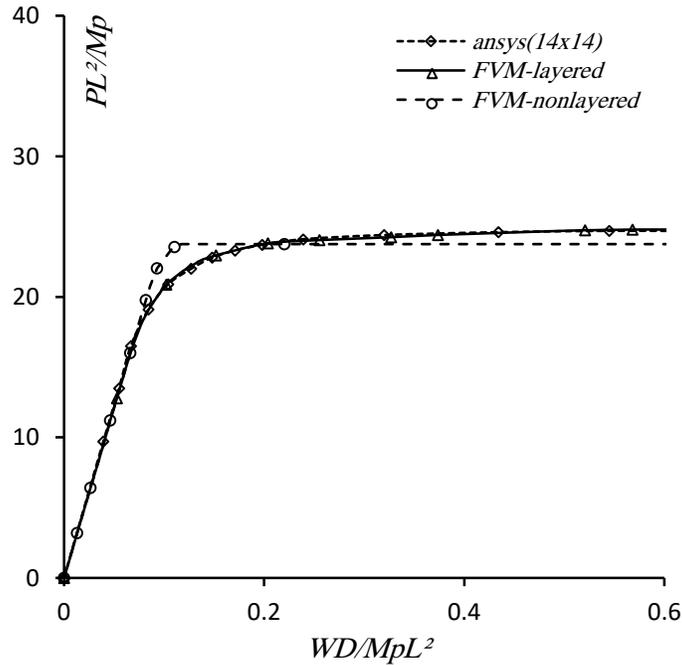
Fig. 6. Load-deflection paths obtained by layered and non-layered approaches for the simply supported plate subjected to a uniformly distributed load
