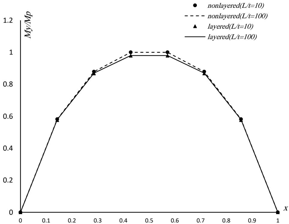
**Fig. 10.** Moment diagram at the middle cross section ( $y = 0.5$ ) corresponding to  $PL^2/M_p = 16$  and different  $L/t$  (simply supported plate subjected to a uniformly distributed load)
