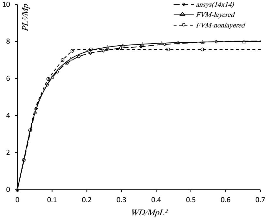
**Fig. 11.** Load-deflection paths obtained by layered and non-layered approaches for the simply supported plate subjected to a concentrated load at the center
