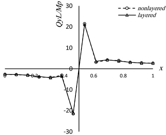
Fig. 13. Shear force diagram at the middle cross section ( $y = 0.5$ ) corresponding to  $PL^2/M_p = 6.5$  (simply supported plate subjected to a concentrated load at the center)
