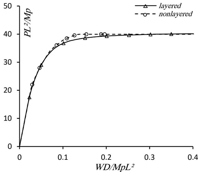
Fig. 14. Load-deflection paths obtained by layered and non-layered approaches for the clamped plate subjected to uniformly distributed load
