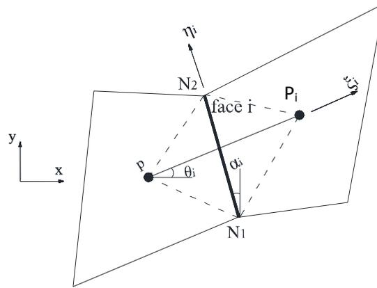
Fig. 2. Two adjacent control volumes on a mesh of elements
