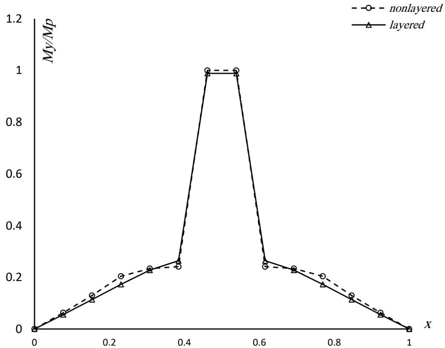
**Fig. 12.** Moment diagram at the middle cross section ( $y = 0.5$ ) corresponding to  $PL^2/M_p = 6.5$  (simply supported plate subjected to a concentrated load at the center)
