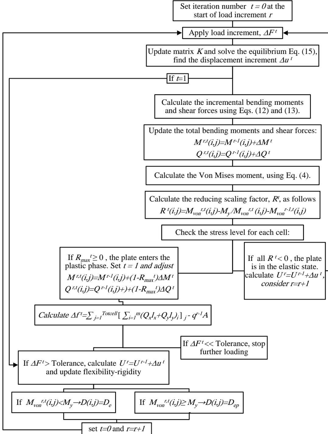
**Fig. 4.** The iterative solution procedure in non-layered approach for the elasto-plastic analysis of Mindlin plates, (Note: it is assumed that  $H' = 0$ )
