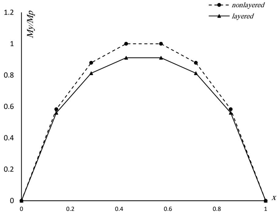
Fig. 8. Moment diagram at the middle cross section ( $y = 0.5$ ) corresponding to  $PL^2/M_p = 20.7$  (simply supported plate subjected to a uniformly distributed load)
