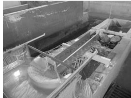
Fig. 4. A view of spillway physical model in scale 1:75
