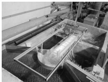
Fig. 5. A view of spillway physical model in scale 1:50
